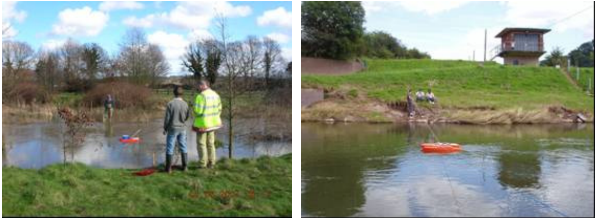
Figure 4.12 ADCP measurements by means of ropeway.
