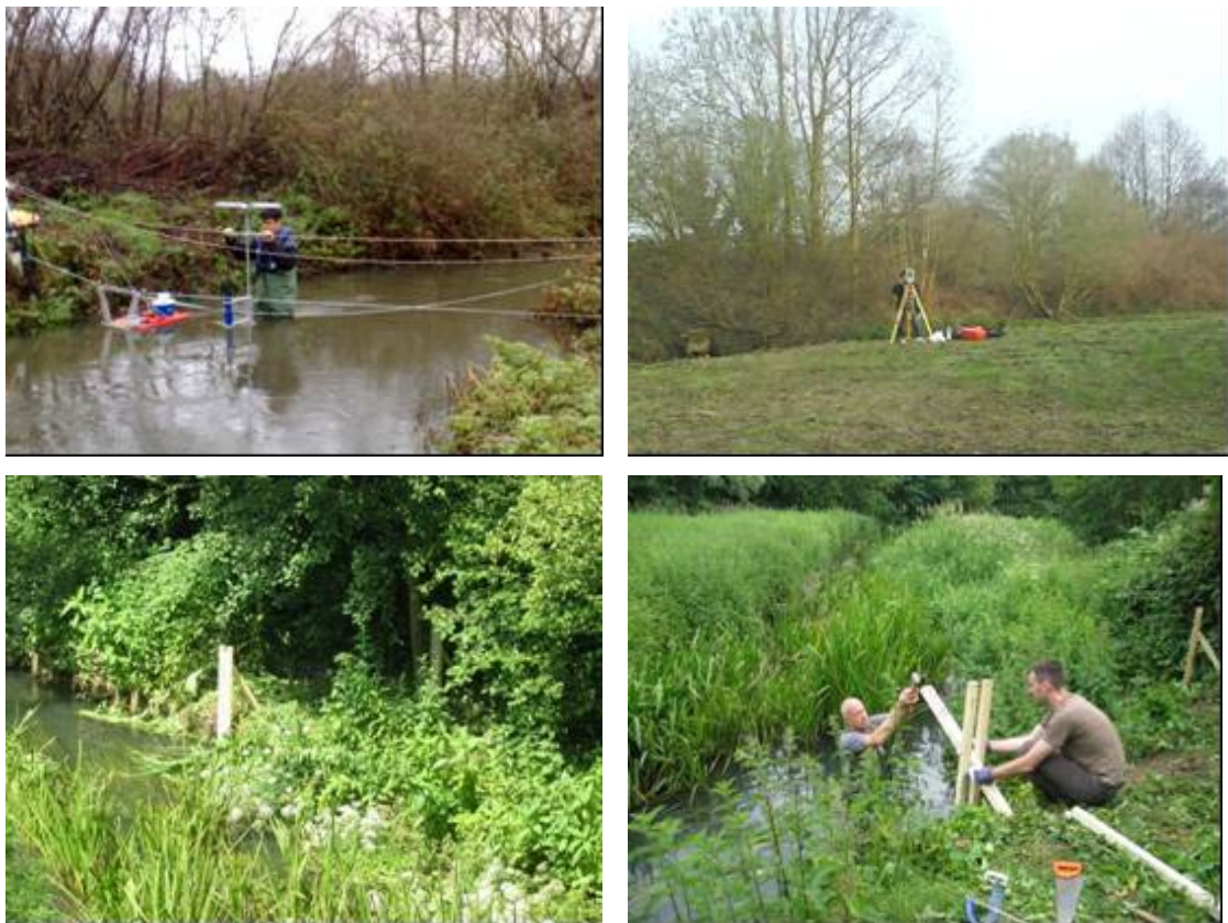
Figure 4.14 Clockwise from top left: total station survey, ADV measurement, staff gauge installation, a staff gauge.
