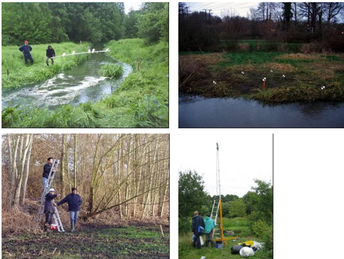
Figure 4.13 Clockwise from top left: seeding for PIV, benchmarks for PIV, video camera attached on a hydraulic pole, video camera recording.
