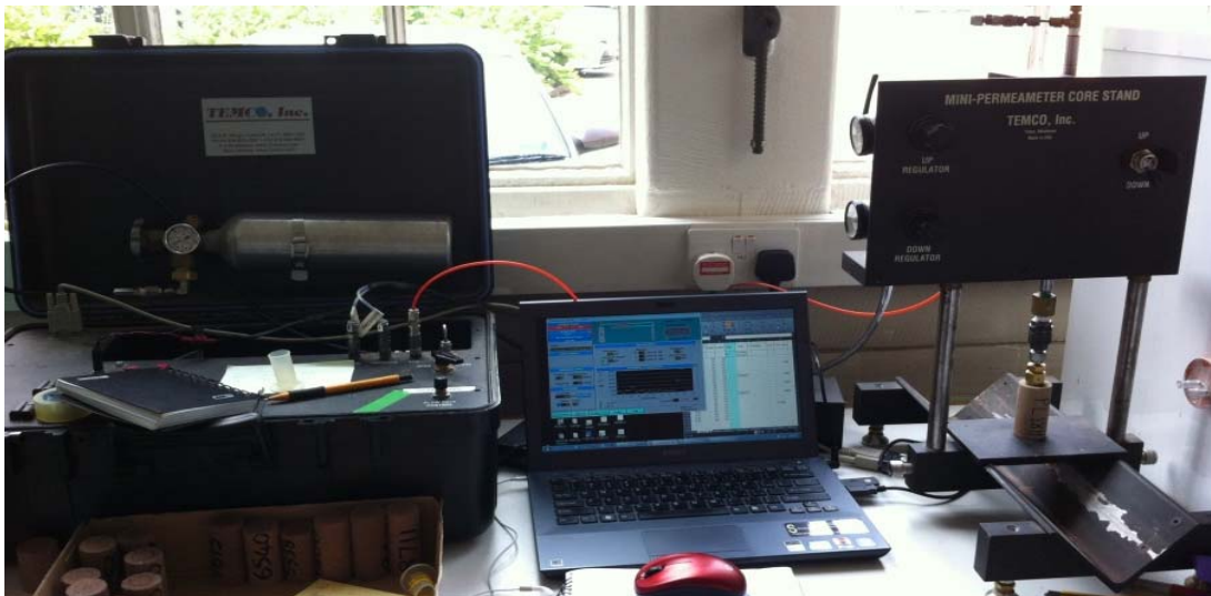
Fig.2-7. A photo of the air probe /mini-permeameter apparatus set up: The Temco Mini-permeameter control box including a compressed gas cylinder (left), a core stand (right), and a computer connect to the system (middle).
