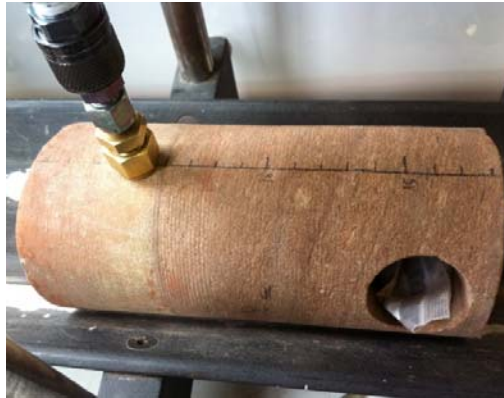
Fig.2-8. Close view of the tip sealing against a core sample.
