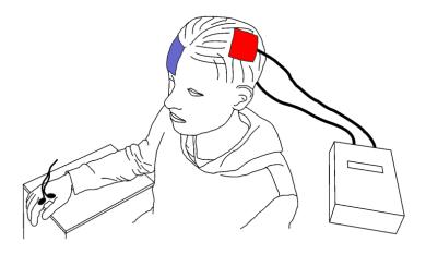
**Figure 8-1:** The experimental setup during tACS stimulation. Participants received 10 min of tACS stimulation with a peakto-peak amplitude of 1 mA. Stimulation was either sham, or at a frequency of 20 or 140 Hz. The anode (red electrode) was placed over the motor hotspot as found with transcranial magnetic stimulation, whilst the cathode (blue electrode) was placed over the contralateral orbit.
