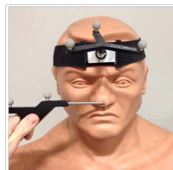
Figure 6. Reflective infrared sphere marked headband and registration wand. In this example, 'Nose Tip' is being registered as a facial landmark.
