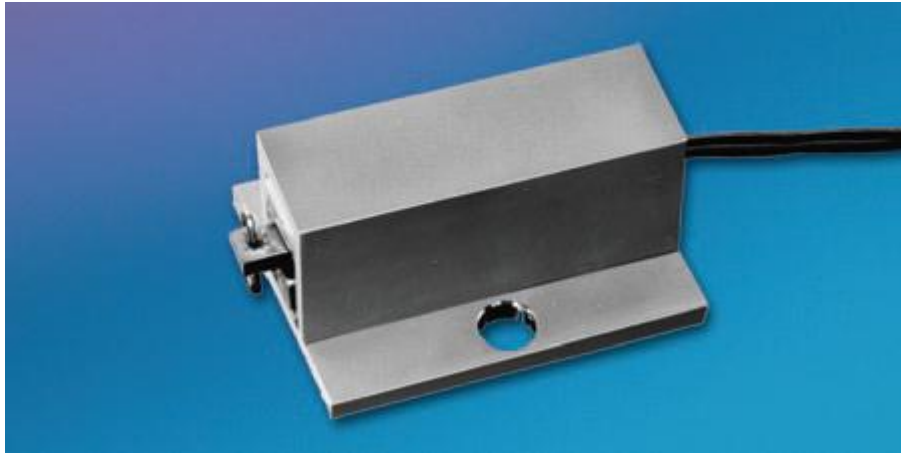
Figure 3.9: BG-1000 force transducer.
