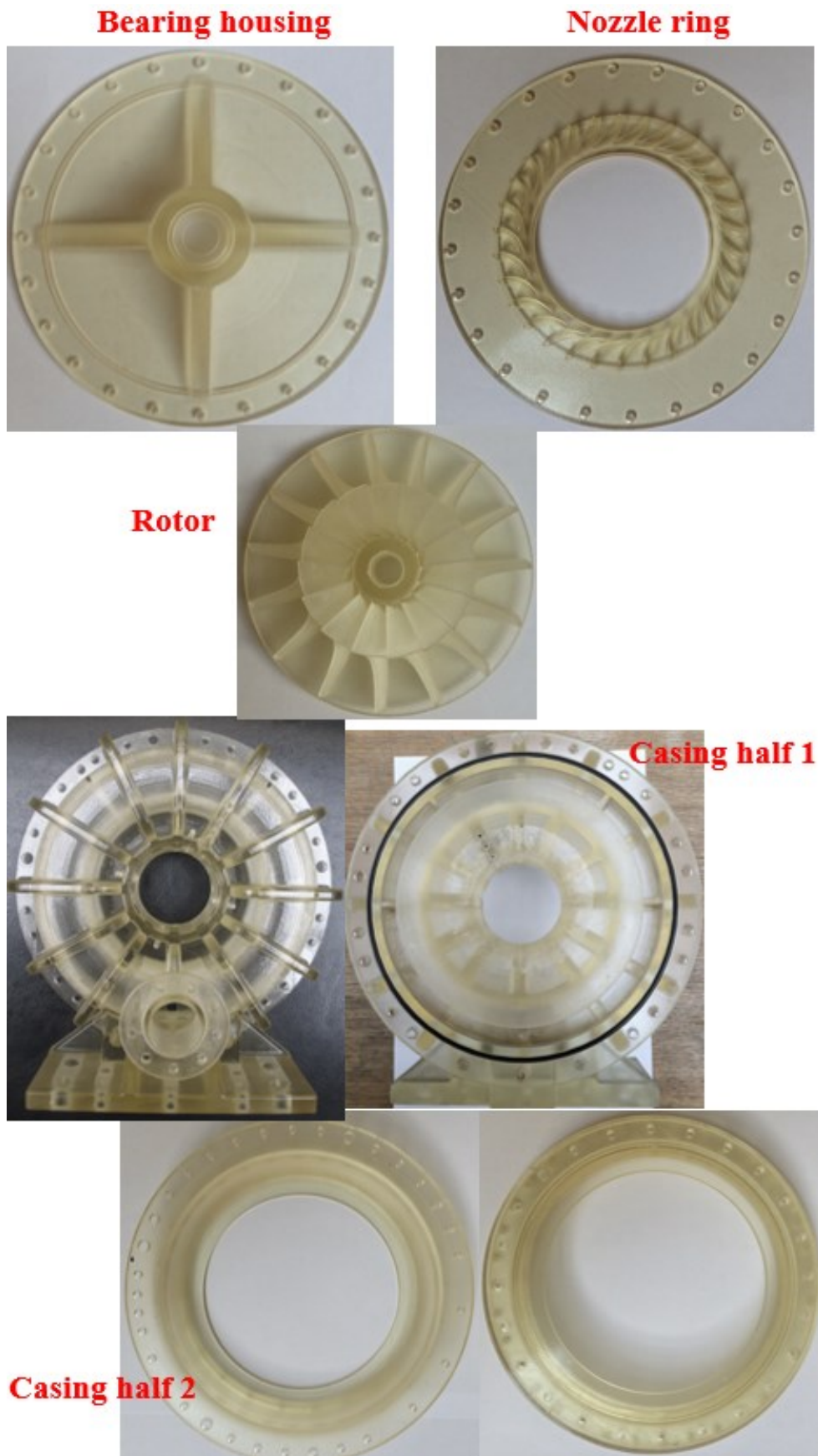
Figure 4-4 Manufactured turbine components with 3-D printing
