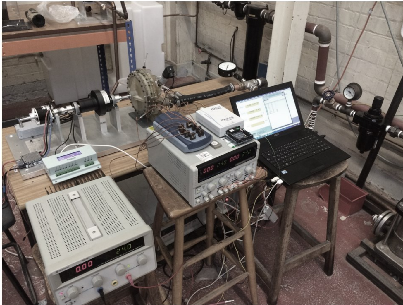
Figure 4-6 Fabricated experimental facility for testing the compressed air RIT
