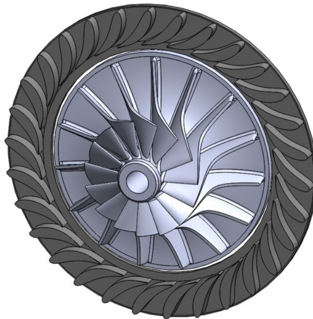
Figure 3-38 Final 3-D geometry of the rotor and nozzle
