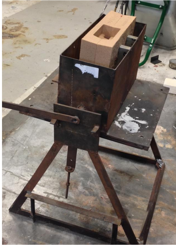
Figure 38 - The frame used to roll the mould over to ensure proper filling
