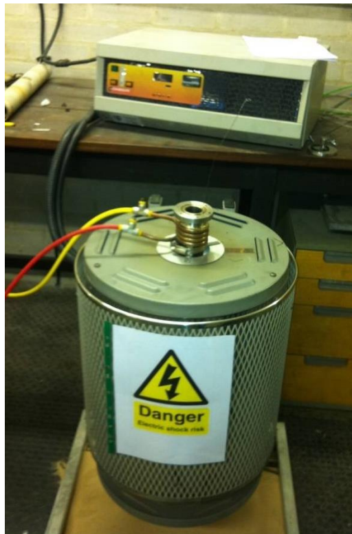
Figure 35 - Cylindrical furnace used to heat the oxidation cell (shown inserted)
