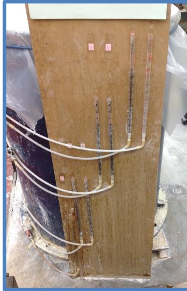
Figure 6.2: Water level measurement tubes and board
