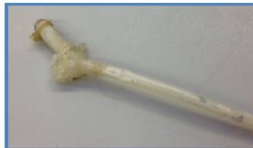
Figure 6.4: Model piezometers used in the large unit cell tests
