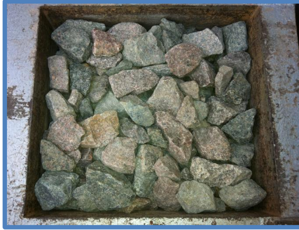
Figure 4.3: Granite (PA) from Tipton site in a large shear box
