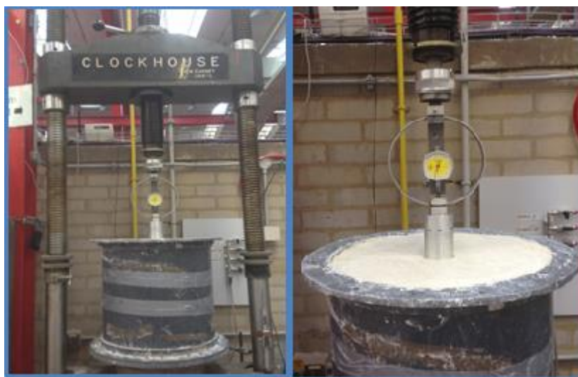
Figure 6.7: Set up for the small unit cell tests
