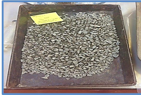
Figure 4.6: Small granite used for the unit cell testing
