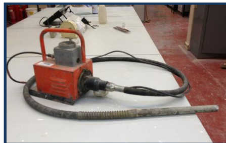
Figure 6.5: Concrete poker used for the compaction of the aggregates during the installation of VSCs
