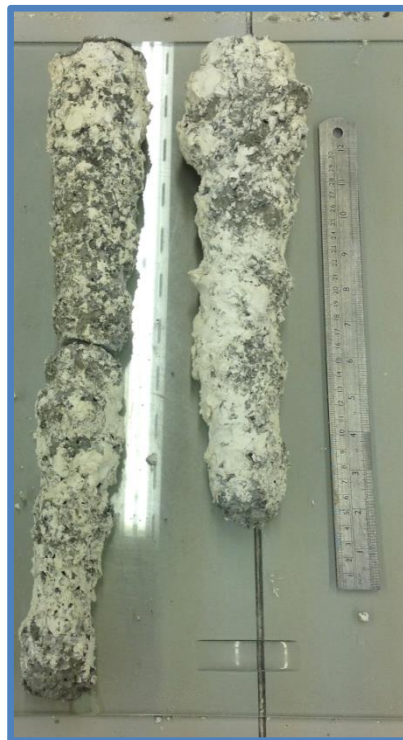
Figure 8.24: Columns contaminated with fines, left to right: the granite contaminated by 10% fines, the granite contaminated by 20% fines
