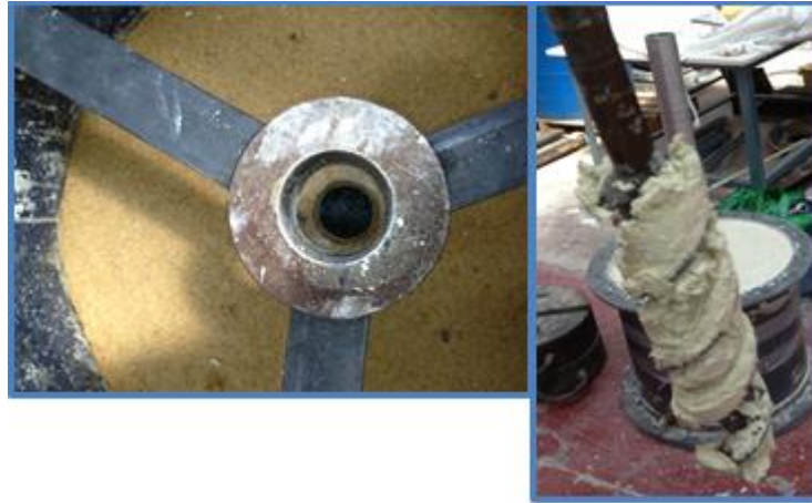
Figure 6.8: shows the cross and the auger used for the column formation
