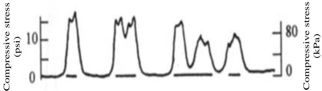
Figure 3.13 Dynamic measurement of subgrade stress (Yoo and Selig, 1979)
