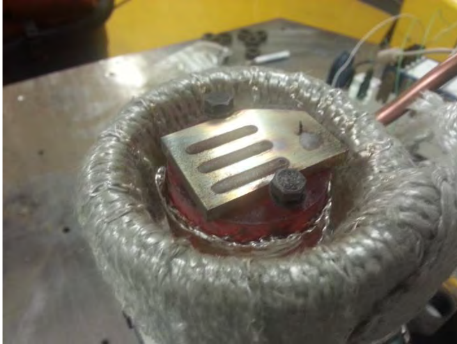
Figure 5-48 - Dilution calibration trial onto preheated CM247LC substrate
