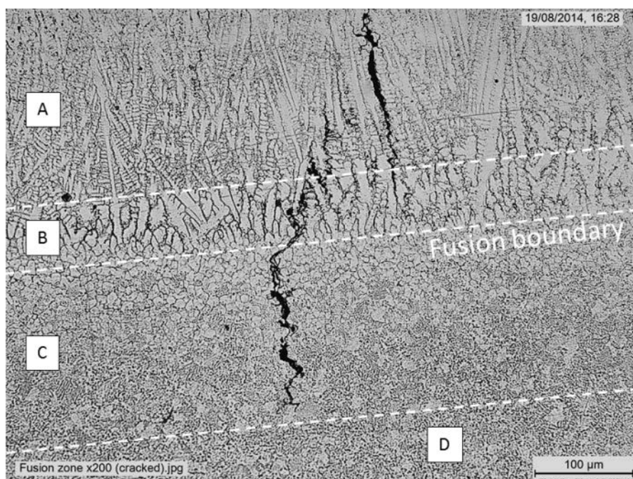
Figure 4-43 - 200X optical micrograph of DOE block 15 (1000W laser power). Areas of interest include the fusion boundary, Dendritic growth region (A), Cellular growth region (B), heat affected zone of substrate (C) and underlying unaffected substrate (D).
