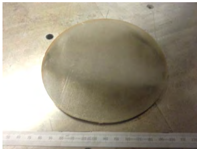
Figure 4-1 - 5mm thick CM247LC substrate in the as-cut condition, cut using the Wire EDM process
