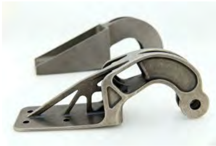
Figure 2-4 - Topologically optimised hinge bracket from an Airbus A380 manufactured using conventional machining (rear) and topologically optimised additive manufacture routes (front)
