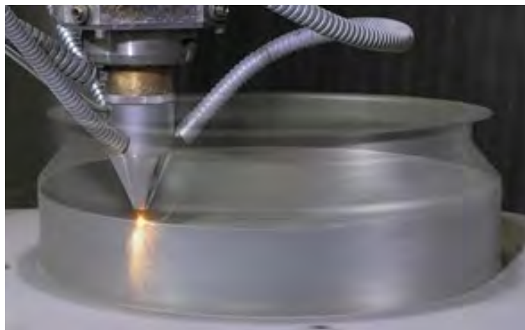
Figure 2-7 - Laser metal deposition manufacture of helicopter engine combustor housing using 5-axis Trumpf DMD machine at TWI Yorkshire [20]
