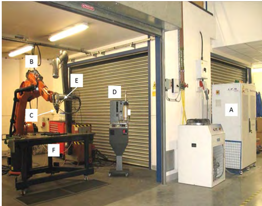
Figure 3-1 - TWI Yorkshire robotic laser processing cell used for deposition trials. A) 7KW IPG fibre laser B) KUKA KR30HA robot C) Coaxial powder delivery nozzle D) Powder feeder E) Laser focusing optics F) Steel welding table
