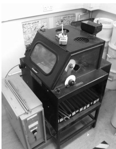
Figure 3:9 Principal of operation of electrostatic separator.
