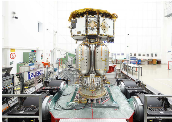
Figure 6.1: ESA's LPF satellite being vibration tested [43]
