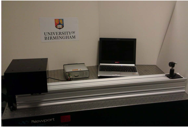
Figure 4.1: Photograph of nEUCLID showing the full target arm and covered optics (the black box), and the electronics box, with a laptop to run the software and for scale.
