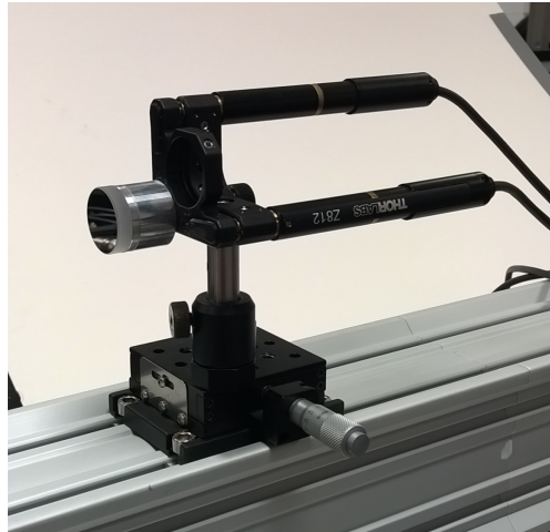
Figure 4.5: Photograph of the nEUCLID target mirror on a DC motor stage, mounted on a micrometer drive and the aluminium rail.
