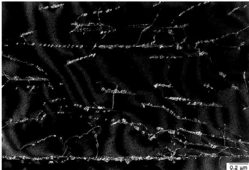
Figure 4.47. Heterogeneous nucleation of precipitates in a sample (Ti-48Al-2Cr) crept at 700 °C, \sigma_a=110 MPa, t=13,400 h to strain \varepsilon=0.46\% [115]
