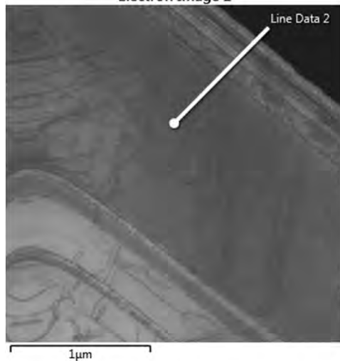
Figure 7.2. TEM foils taken from the fracture surface of specimenS tested at 700 °C with an R ratio of 0.8: (a) the fracture surface taken along crack growth direction, (b) two sites where the TEM foils were taken, and results of oxidation analysis of site 1 and 2
