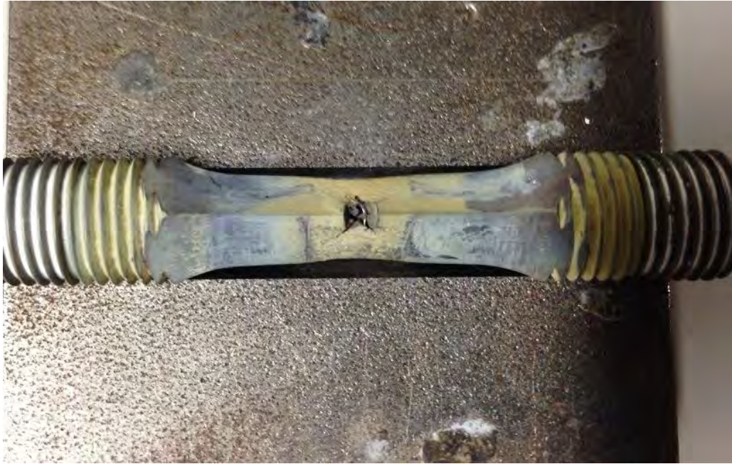
Figure 6.59. Specimen CC009 from TIMET 3 rd batch failed due to creep, severe deformation can be observed around the widely opened crack
