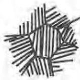
Figure 4.3. Schematic of microstructure categories in gamma TiAl-based alloys
