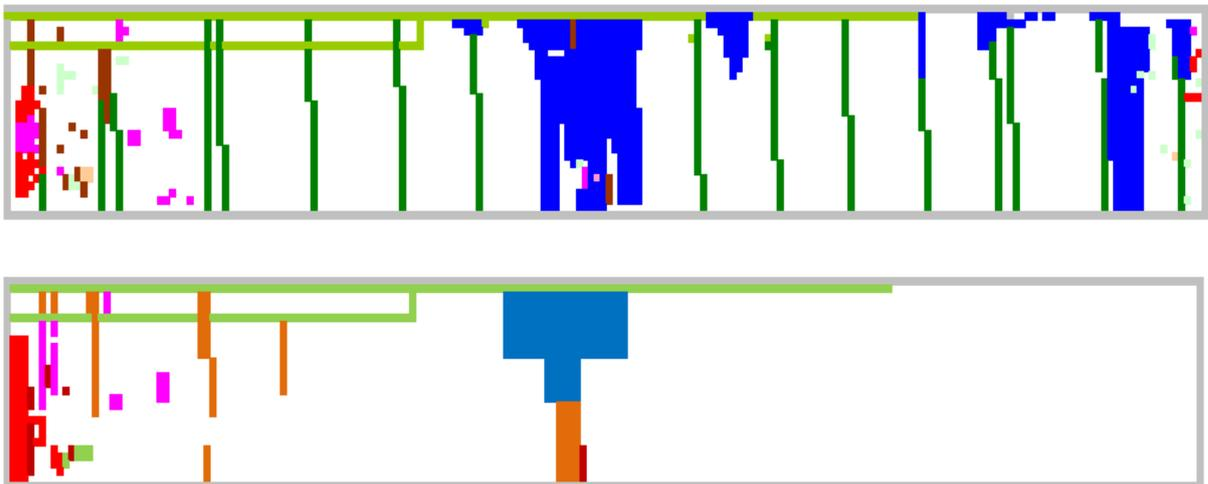
**Figure 101: Defect maps produced by IBIS (top), and on-site inspection (bottom). Site (f), west abutment.**
