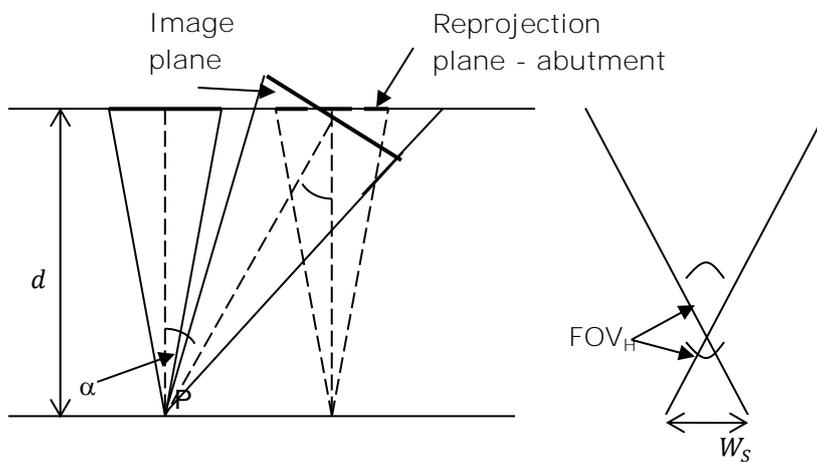
**Figure 84: Illustration of some of the concepts and angles involved in image reprojection.**
