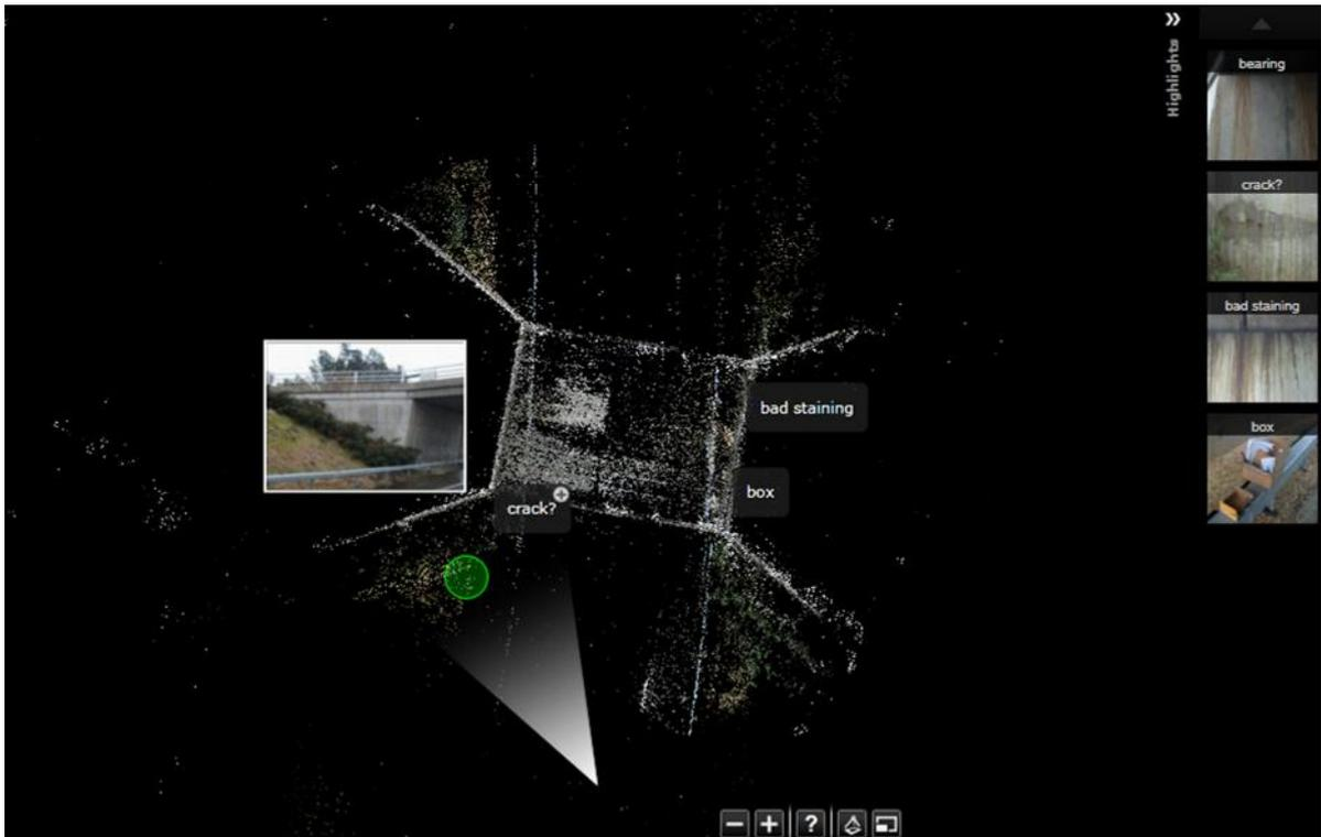
**Figure 71: Point cloud of bridge showing a selection of 'highlight' views.**
