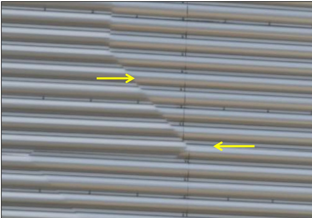
**Figure 66: Panoramic image created using GigaPan Stitcher, showing misalignment of image features.**
