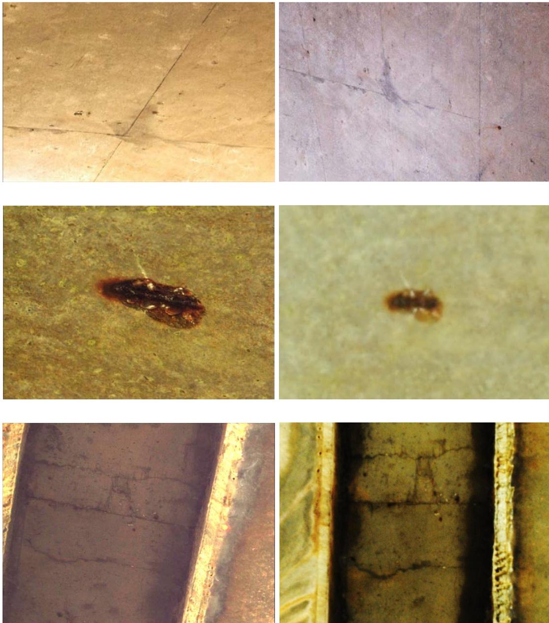
**Figure 52: Example images taken using the ScanSites CR system (left) and traditionally collected images at 1 pixel per mm of the same locations.**
