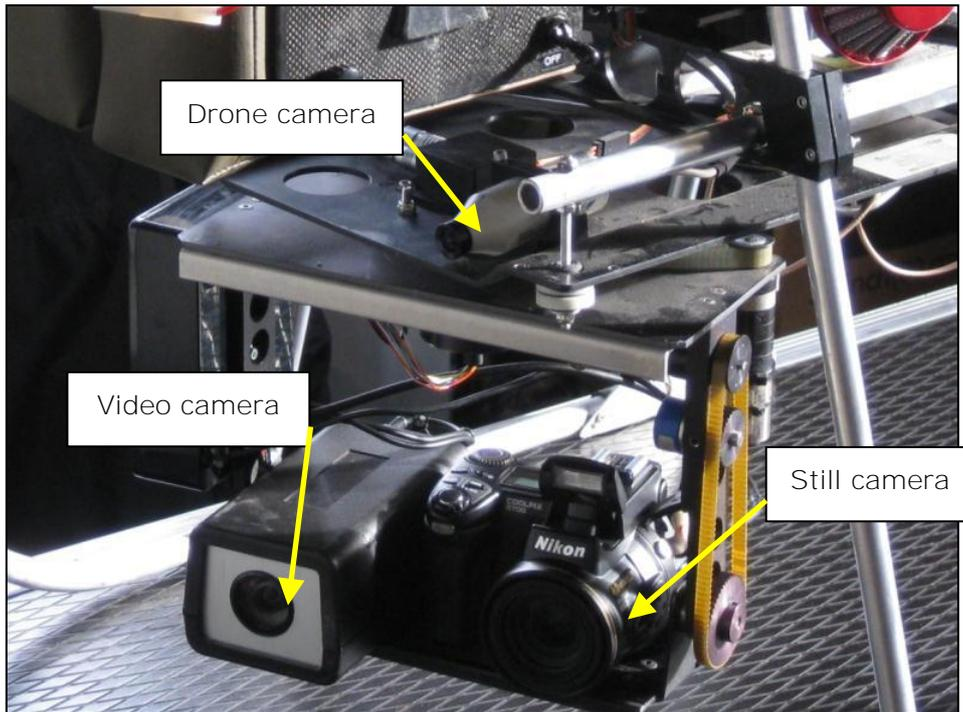
**Figure 62: Inspection camera and still camera mounted on gyrostabilised turret.**
