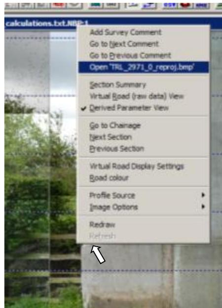
Selecting the **Open 'image\_file\_name.bmp'** option will open a new window in another application (usually Windows Picture and Fax Viewer) where the individual image can be inspected.
