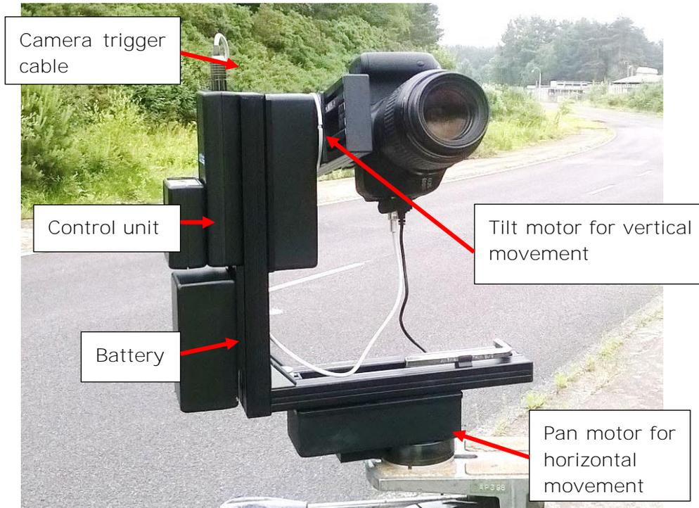
**Figure 74: Clauss Rodeon ST with camera fitted.**
