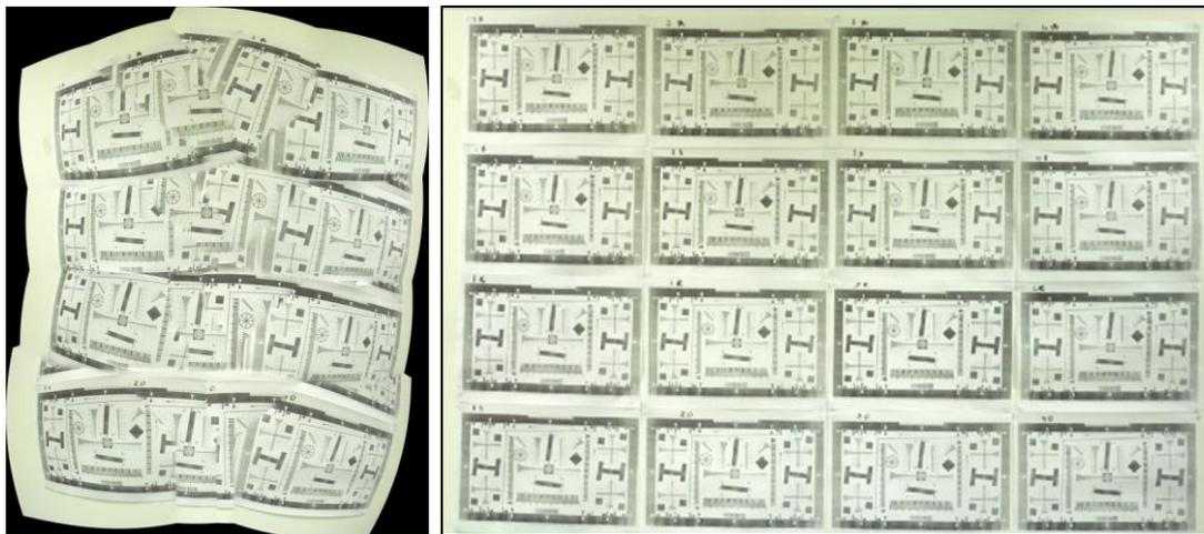
**Figure 69: Result of stitching together 16 individual images of test targets using GigaPan Stitcher software (left) and Microsoft ICE.**
