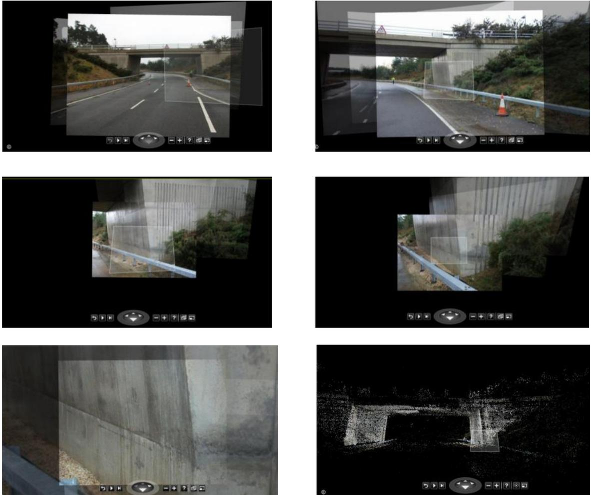
**Figure 70: Series of images, displayed in Photosynth browser window, moving progressively closer to part of east end of north abutment. Also shown is the point cloud of the bridge.**
