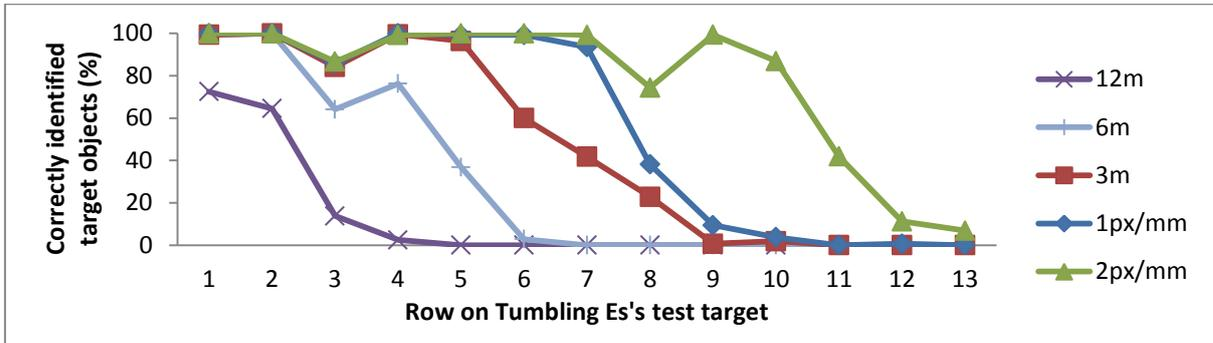
**Figure 48: POD of test objects of different sizes on chart E<sub>A</sub> at 12m, 6m, 3m, and in images at 1 pixel per mm and 2 pixels per mm.**
