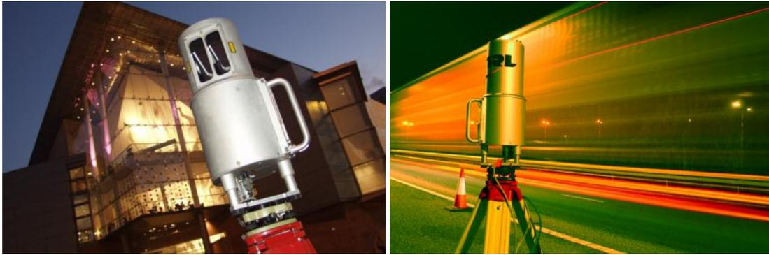
**Figure 54: Riegl LMS-Z360i laser scanner as operated by TRL.**
