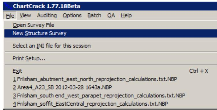
This will open a survey of a fixed face size (50m wide by 20m high) on which to overlay a set of images. To load the images you must open them manually by selecting the “**Open Downward Image Files**” button, shown below.
