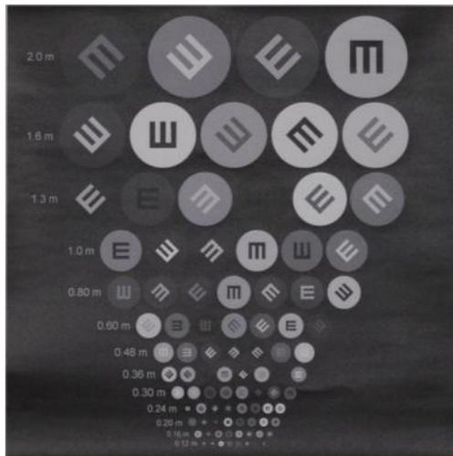
Figure 40: Tumbling E's chart with varying object-background contrast ratios ( $E_A$ ).
