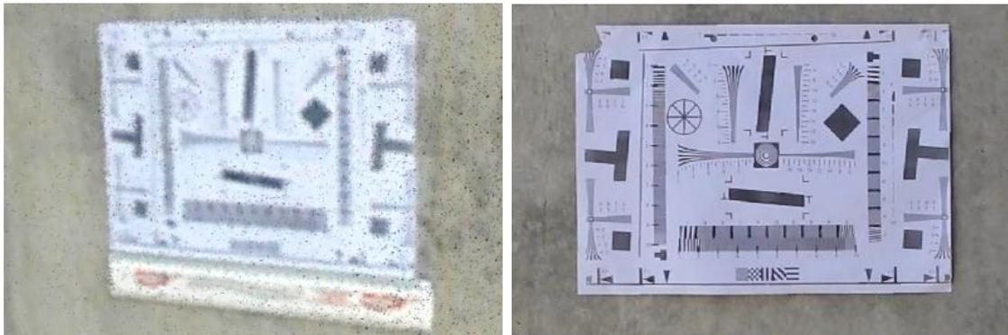
**Figure 60: Enlarged view of the high resolution scan data for the target fixed to the abutment (left), and image showing same target at 1mm per pixel.**
