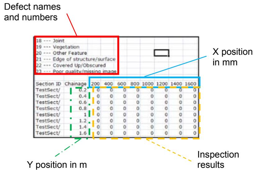
**Figure 95: Example of data produced by inspection software, used to create defect maps.**
