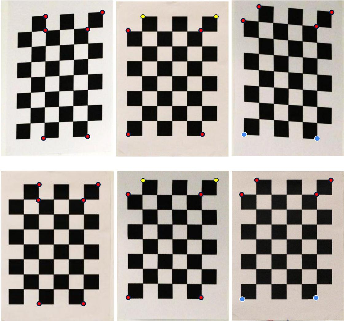
**Figure 109: Examples of images before (top) and after (bottom) reprojection to remove perspective effects.**
