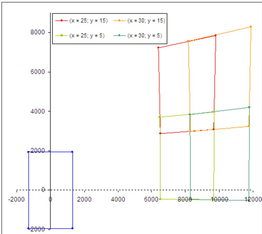
**Figure 83: Illustration of how viewing angle can affect size and shape of view represented in image.**
