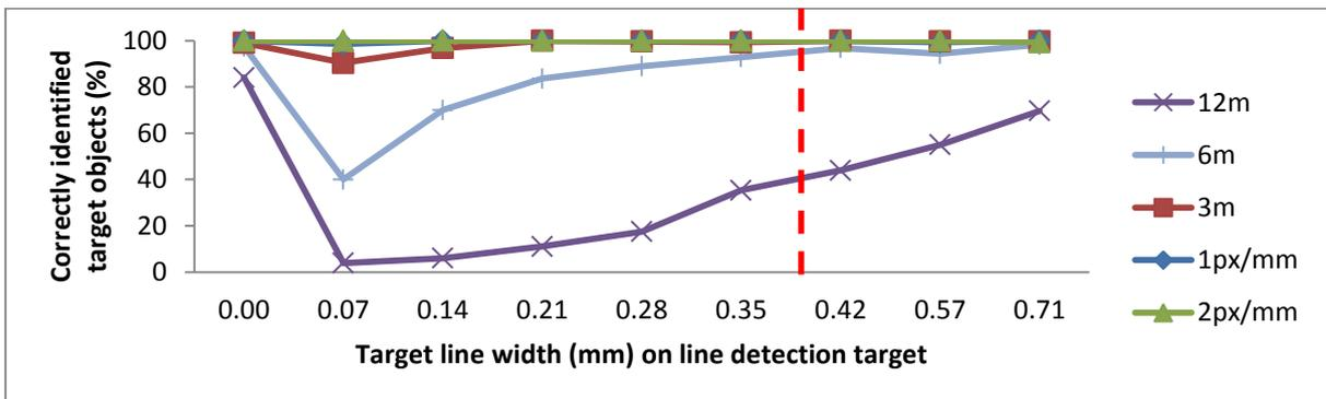
**Figure 49: POD of test objects of different widths on chart T<sub>A</sub> at 12m, 6m, 3m, and in images at 1 pixel per mm and 2 pixels per mm.**
