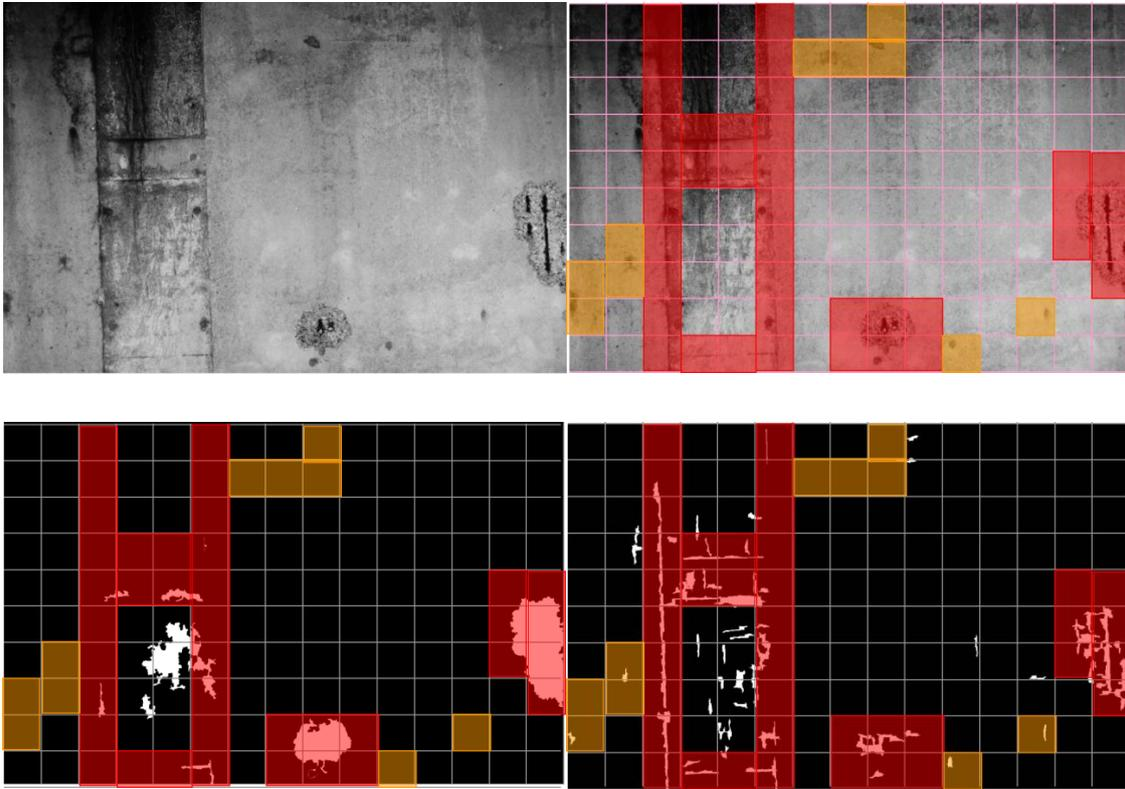
**Figure 117: Examples of IBIS images following application of various image processing techniques (segmentations based on image entropy and on concentration of detected edges) compared against manually generated reference data showing which cells contain features or defects.**
