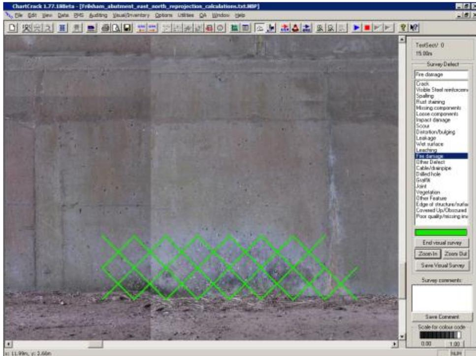
The following summarises different ways of recording defects and removing defects when incorrectly marked
