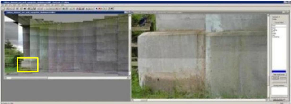
**Figure 93: Screenshot of image-based inspection software showing zoomed out thumbnail view, and detailed section of images.**
