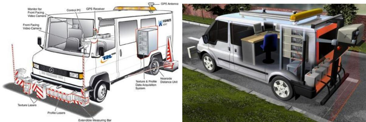
**Figure 31: HARRIS1 and HARRIS2 vehicles, developed and operated by TRL on behalf of the Highways Agency.**
