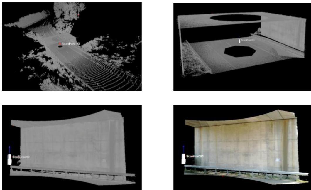
**Figure 56: The scan data obtained from a single position in different stages of post-processing. Scan position was directly under the bridge approximately in the centre of the road.**
