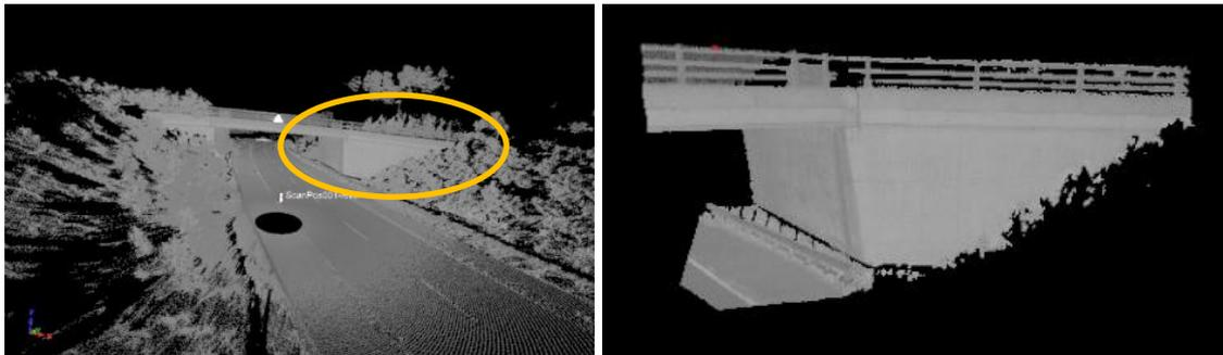
**Figure 55: Full data collected using scanner at Scan position 1 (left) and following cleaning process to remove extraneous data (right).**
