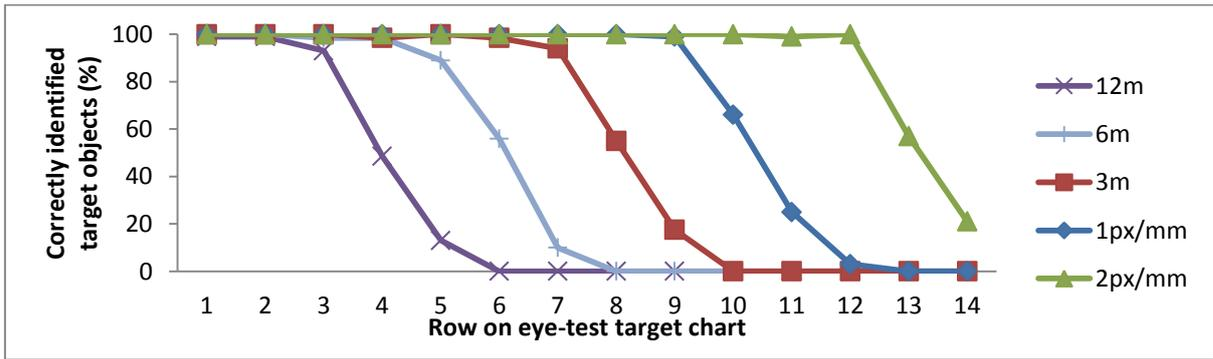
**Figure 47: POD of test objects of different sizes on chart L<sub>B</sub> at 12m, 6m, 3m, and in images at 1 pixel per mm and 2 pixels per mm.**
