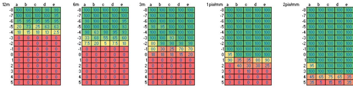
**Figure 46: Detection rates of each individual test object on chart L<sub>B</sub> at (from left) 12m, 6m, 3m, and in images at 1 pixel per mm and 2 pixels per mm.**
