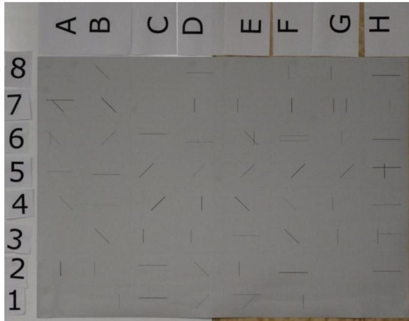
**Figure 41: Array of lines of known thickness and orientations ( $T_A$ ).**
