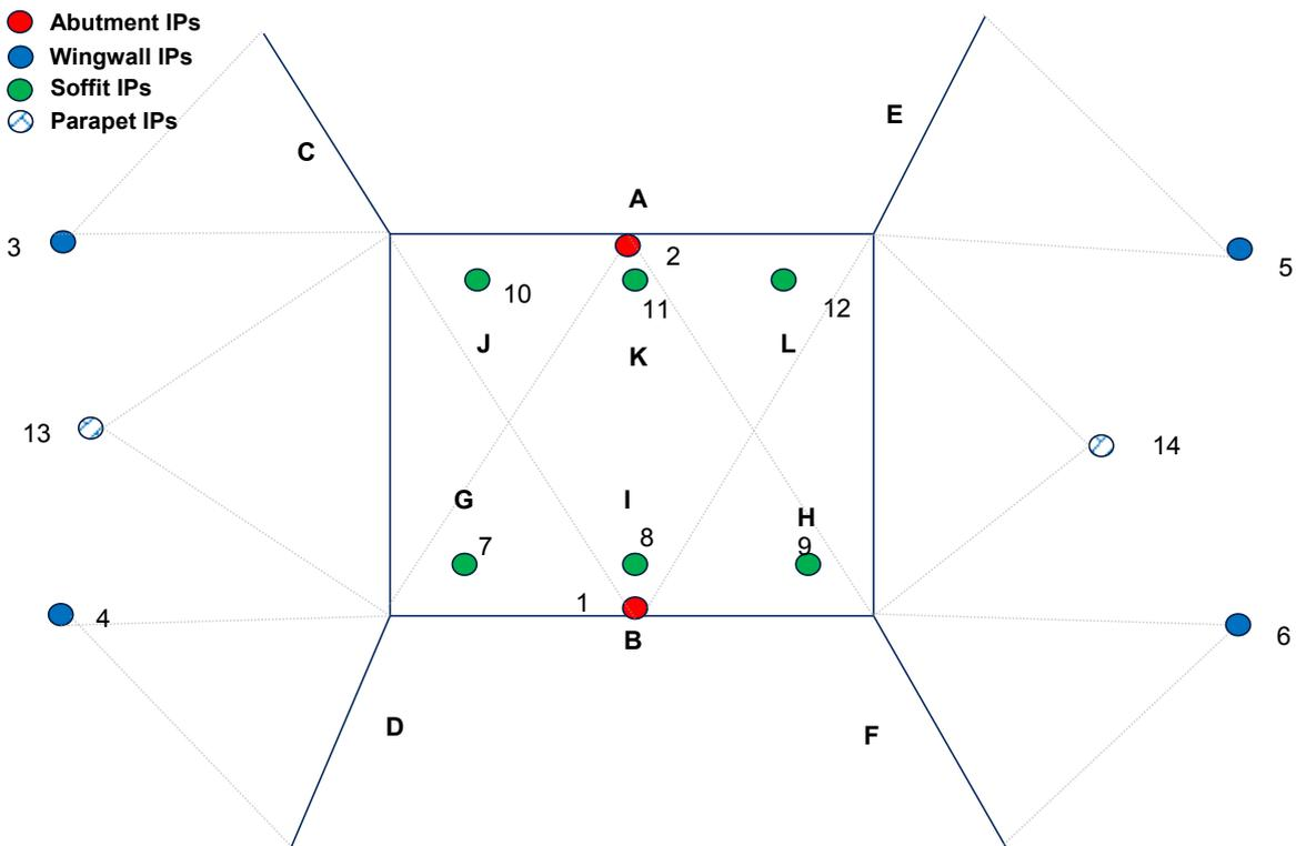
**Figure 78: Imaging positions for IBIS.**
