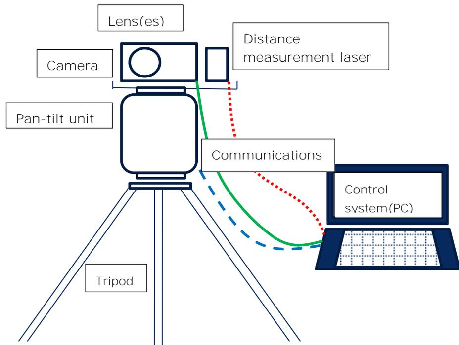
**Figure 72: Schematic drawing of elements of system hardware.**
