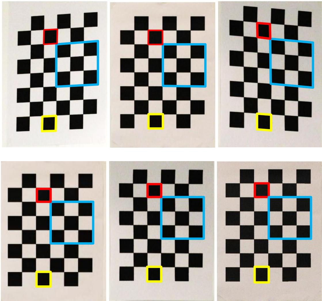
**Figure 110: Examples of images before (top) and after (bottom) reprojection showing squares used in measurement of pixel size.**
