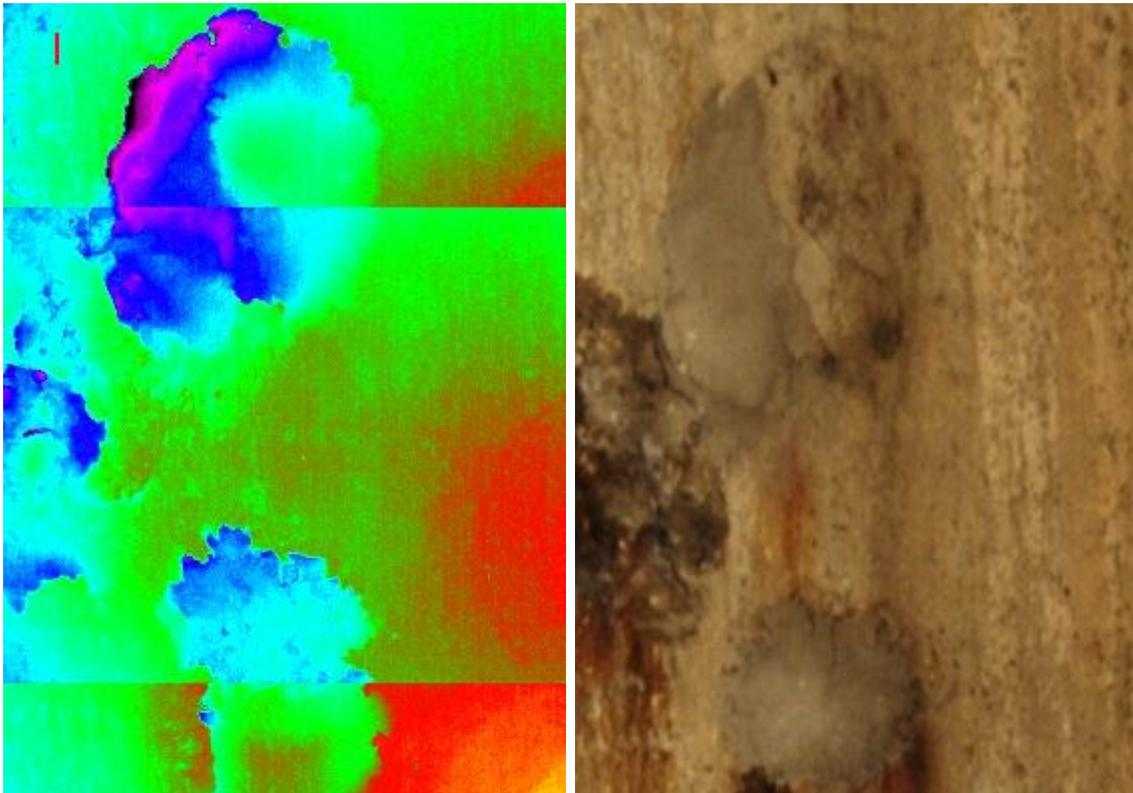
**Figure 116: Example of thermal and visible images of part of a bridge showing different temperatures on defective and repaired areas.**
