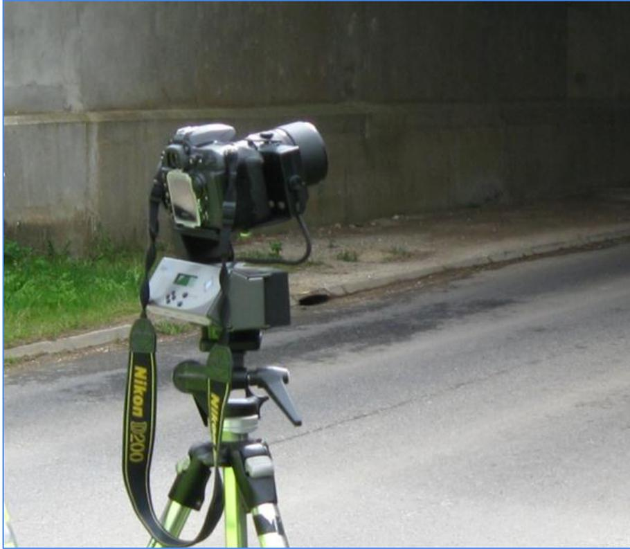
**Figure 73: Prototype image collection system showing camera mounted on GigaPan automated pan-tilt unit.**
