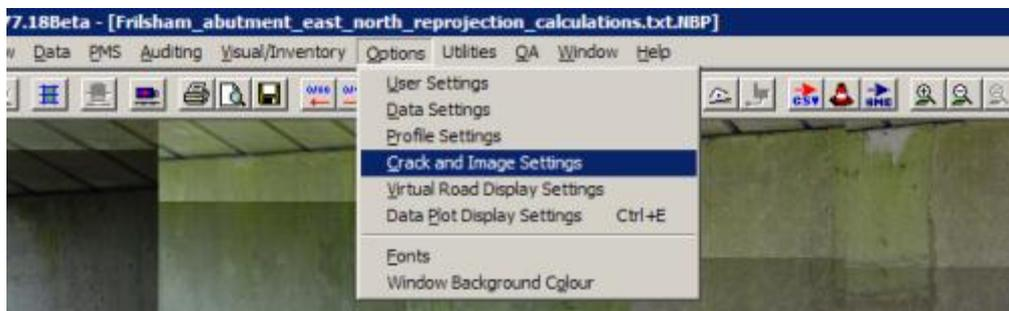
This will bring up the following dialog. Select the "H2/Generic Images" tab, and set the Generic Images **Pixel X Length** and **Pixel Y Length** values. In this example they are set to x=1 and y=1 (shown below), which tells ChartCrack that each pixel covers 1mm in the x direction and 1mm in the y direction on the surface of the structure.
