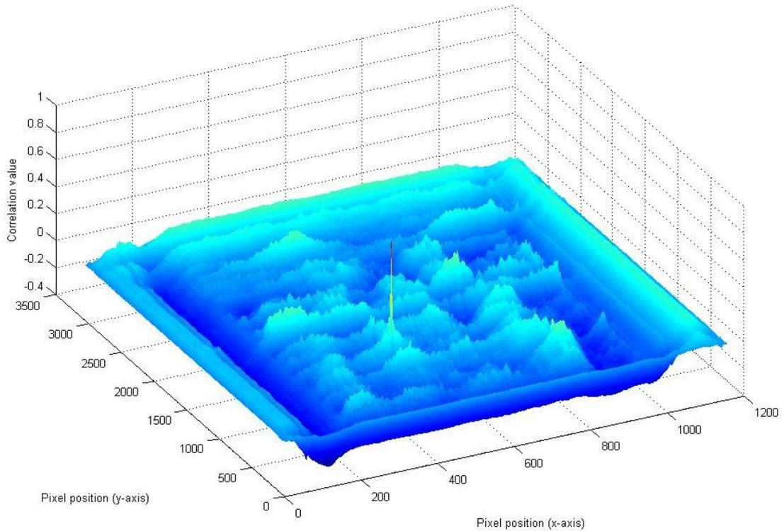
**Figure 88: Correlation coefficients calculated by cross correlating one of the sub-regions shown in Figure 87 with the locked image (peak value at (430,1411)).**
