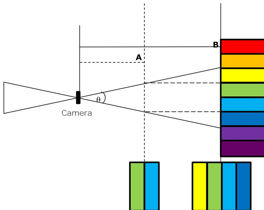
**Figure 34: Demonstration of effect of imaging distance on area imaged.**
