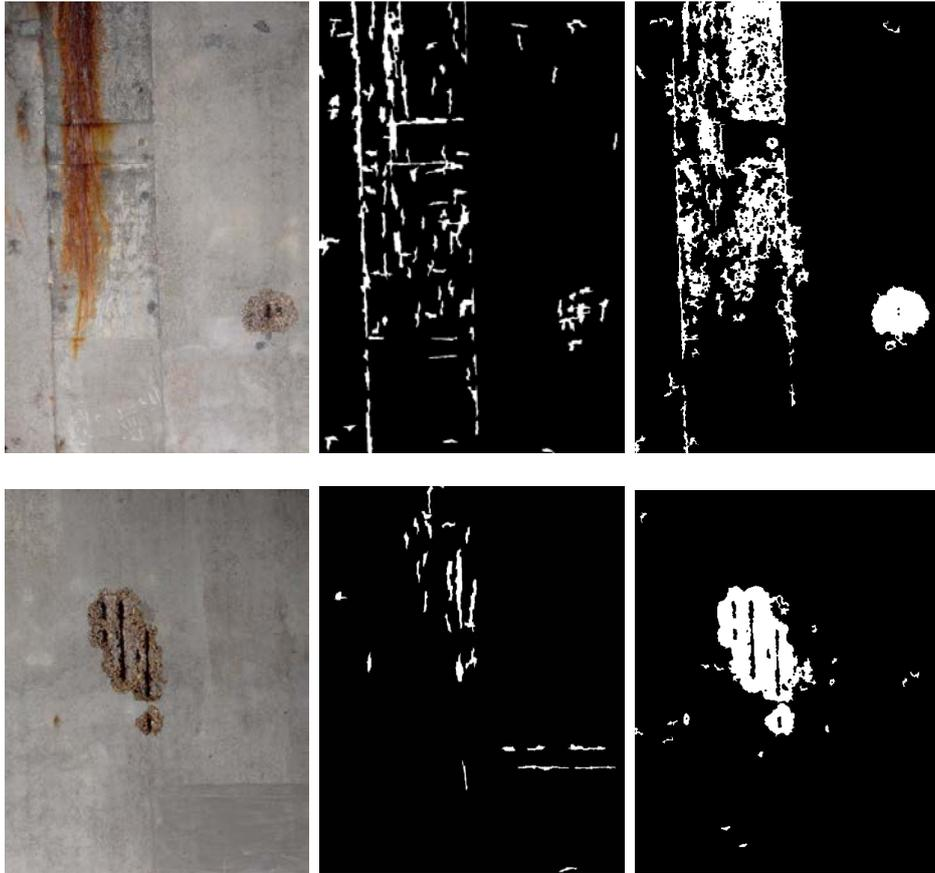
**Figure 115: Example IBIS images following different image processing techniques.**
