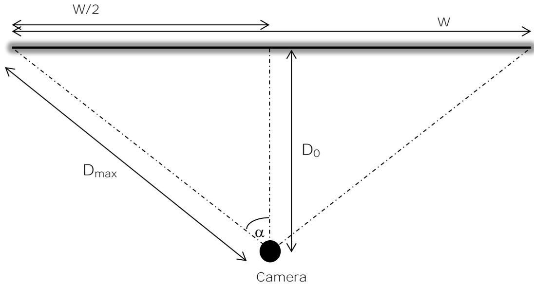
**Figure 77: Change in camera-object distance with changing orientation.**
