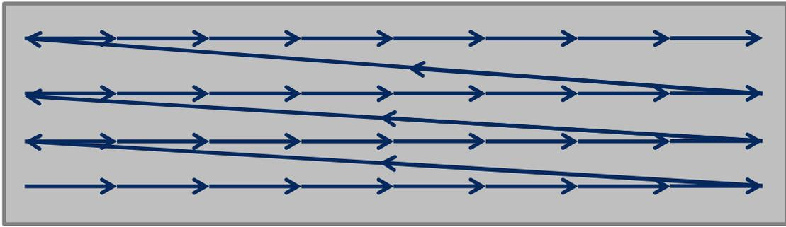
**Figure 79: Image collection path taken by Rodeon ST during collection of scene data.**
