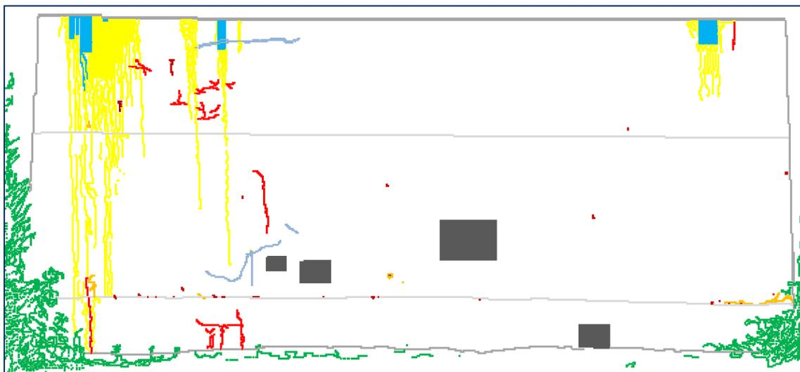
**Figure 96: Example of defect map produced using ChartCrack, overlaid on images (top) and in spreadsheet form (bottom).**
