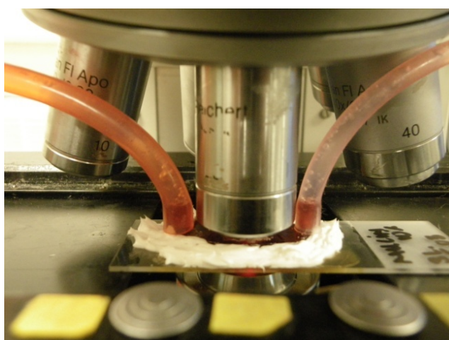
Figure 7.3: Setup for flow cell analysis with Reichert-Jung microscope using 25x magnification lens.
