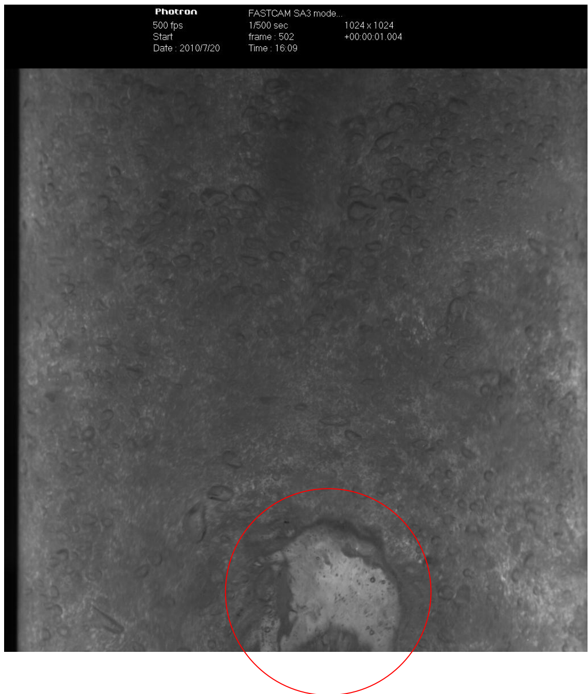
Figure 4.4 Image of heterogeneous flow of air-water column for flow visualisation experiment 2; superficial gas velocity 6.1 cm/s, 1 kg of dissolved sodium chloride. Internal column diameter of 144 mm. TIFF image belongs to file flow_vis_ext_2.avi.
