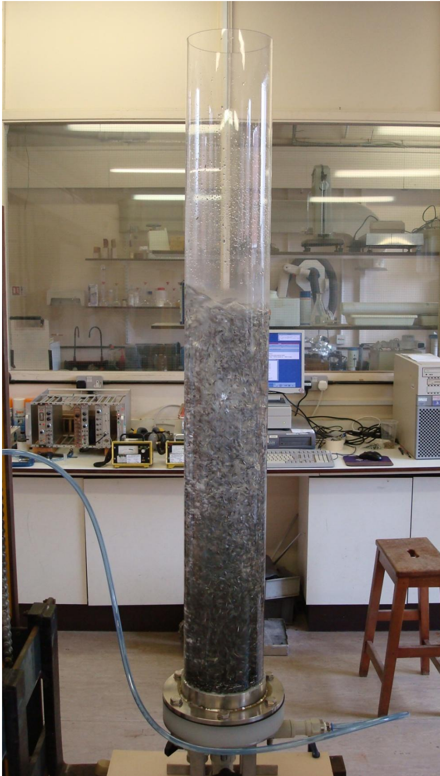
Figure 4.14 A photograph of heterogeneous flow within the air-water-swarf column prior to PEPT experiments.
