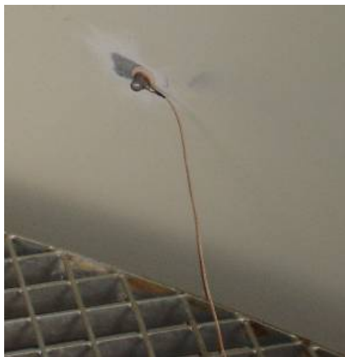
Figure 5.3: Industrial piezoelectric accelerometer used for vibration analysis measurements of an in-service wind turbine tower. The photograph is courtesy of Dr Frederik Vermeulen.
