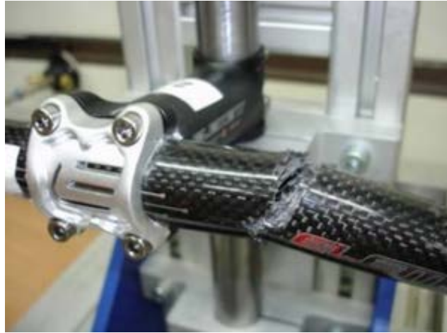
Figure 3.7: Failure of a CFRP component used in bicycles following fatigue testing (the photograph is courtesy of Mr Markus Schatz) [81].
