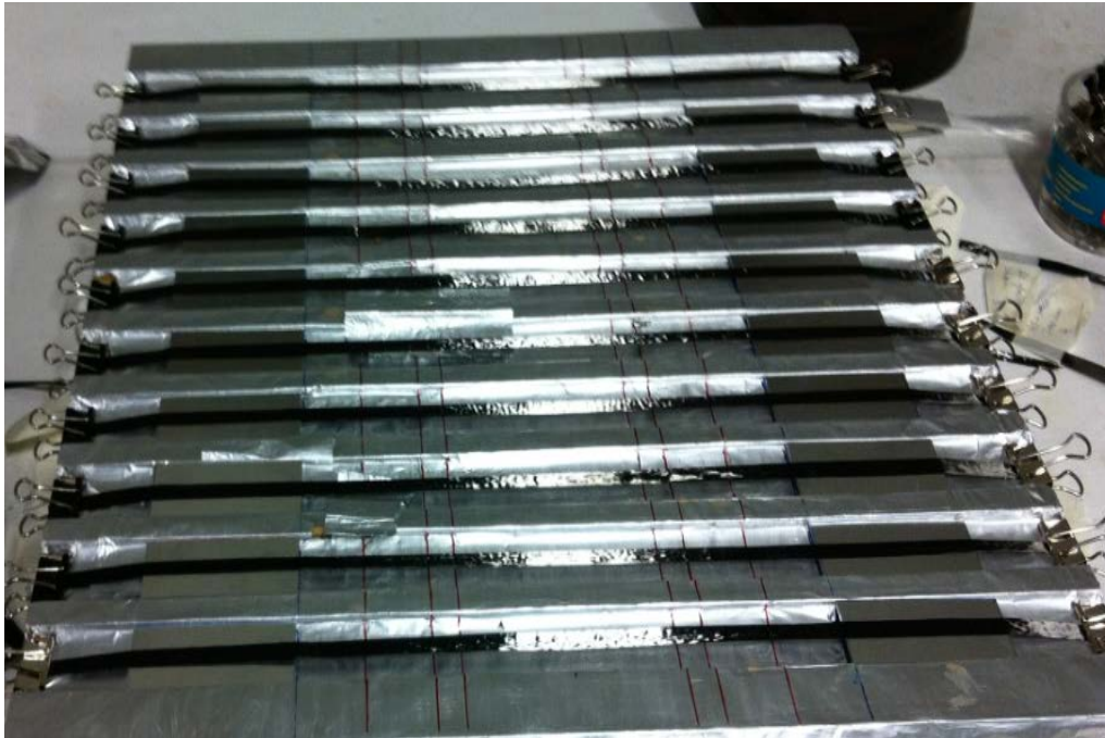
Figure 6.1: Carbon fibre bundles being end-tabbed using aluminium sheets on either side glued together using Scotch-weld.
