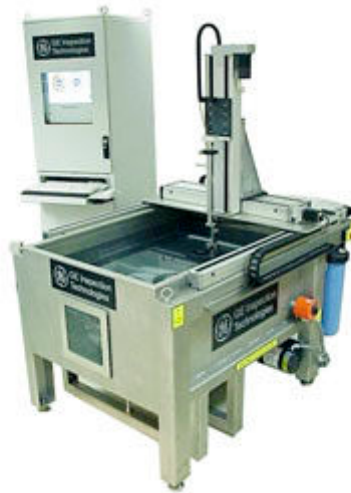
Figure 4.3: Typical immersion tank with automatic manipulator for moving the UT transducer.
