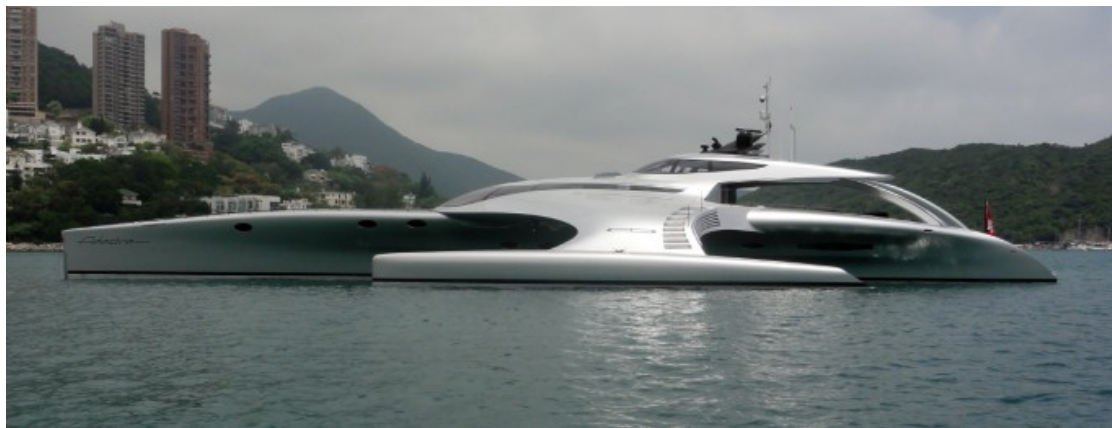
Figure 1.4: The 42.5-metre trimaran motor yacht Adastra made almost entirely of FRP materials. The photograph is courtesy of McConaghy Boats.
