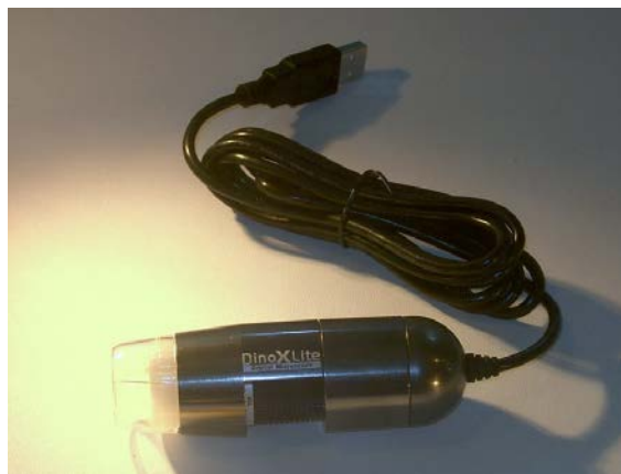
Figure 4.1: Photograph of digital USB optical microscope (the photograph is courtesy of Mr. Rico Shen).
