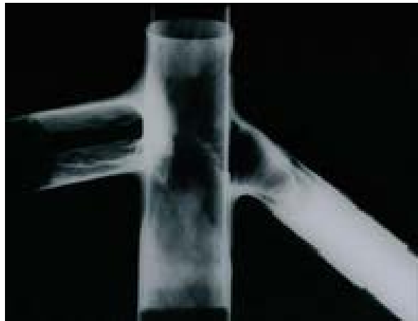
Figure 4.6: Digital radiograph showing extensive damage in a CFRC bicycle component due to fatigue. The radiograph is courtesy of Mr. M. Schatz [81].
