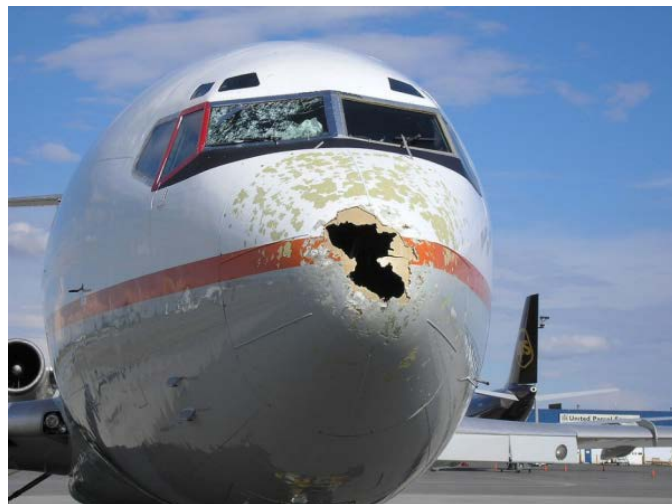
Figure 3.5: Impact damage resulting in failure of the nose of an aircraft (photograph is courtesy of the Centre for Nondestructive evaluation of the Iowa State University) [79].
