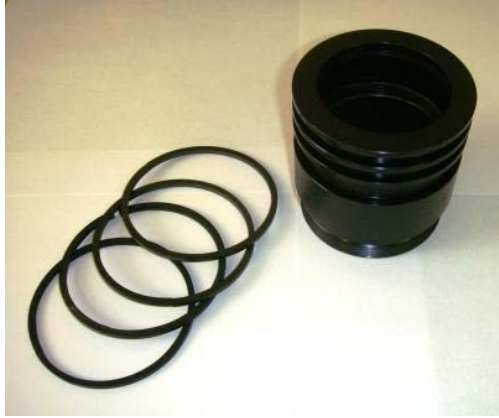
Figure 3-11: Optical engine piston and full stroke transparent optical liner on the single cylinder engine
