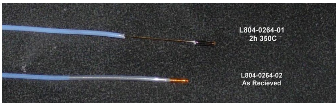
Figure 2.20: OpSens fibre optic probe before and after 2 hours at 350°C under 7 bar hydrogen atmosphere
