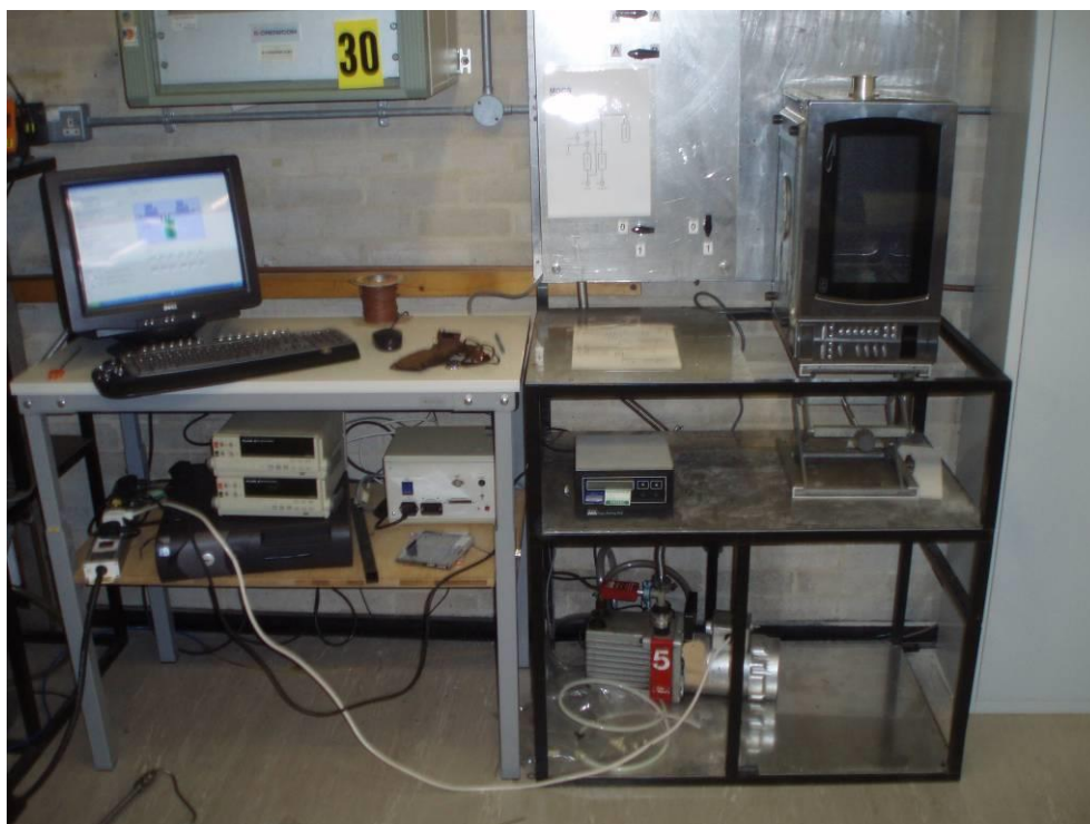
Figure 2.15: Microwave system with gas control board at the University of Birmingham, with vacuum system control and logging computer and the adapted multimode microwave system.
