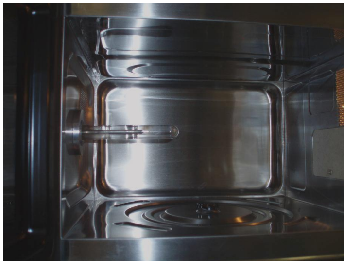
Figure 2.5: Silica sample tube positioned in the multimode domestic microwave cavity
