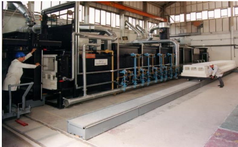
Figure 2.2: Industrial tunnel kiln developed to process 1m 3 of product per hour[117, 118]
