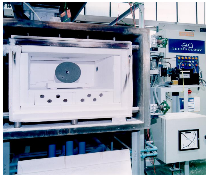
Figure 2.1: Gas heated lab scale hybrid microwave furnace, using mixed mode microwave system from 3 microwave sources[101, 116].
