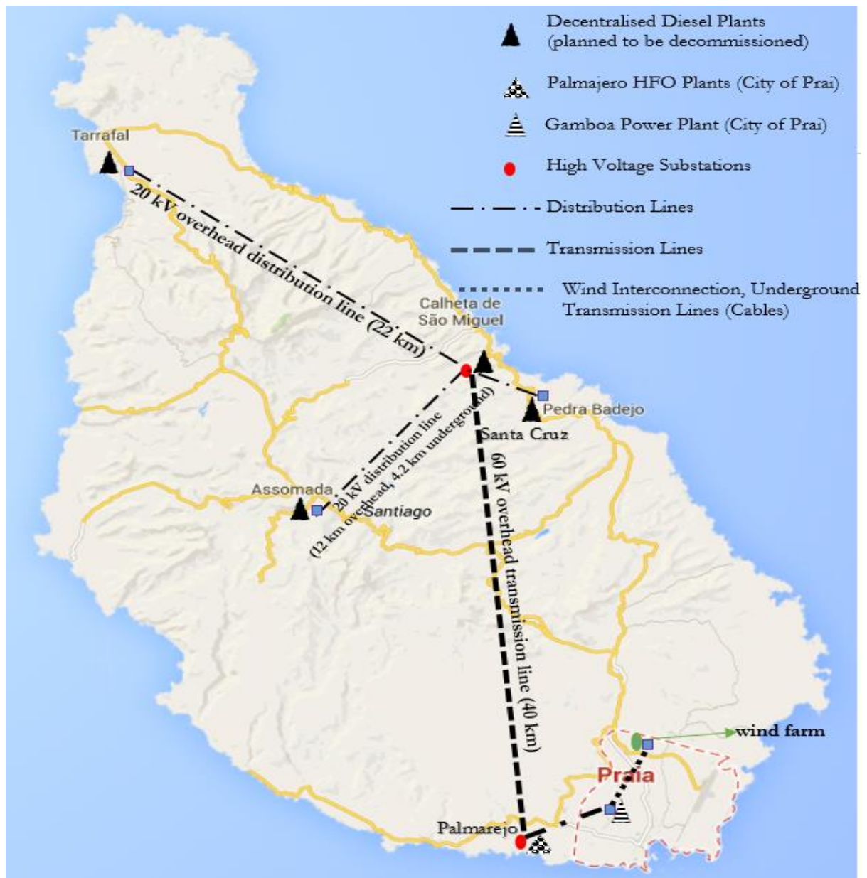
Figure 1.1. Santiago Island of Cape-Verde Energy Network 27
