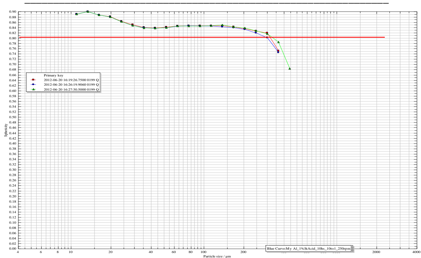
Figure 4. 4 Sphericity graph for Microcrystalline Cellulose particles obtained from a QICPIC Image Analyser (triplicate runs).
