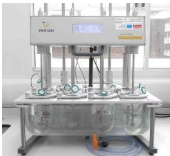
Figure 3. 12 Dissolution apparatus using a basket method
