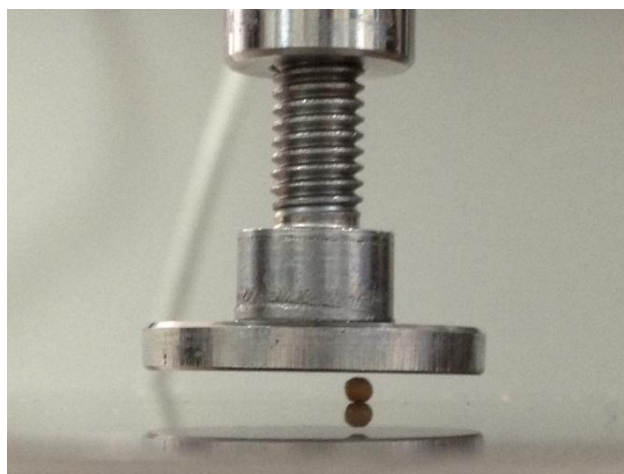
Figure 3. 11 Compression of single dried yeast granule using a Zwick/Roell Z030 mechanical tester
