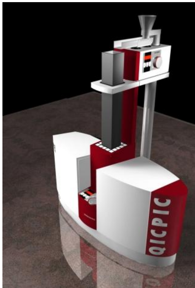
Figure 3. 5 Particle size and shape analyser (Qicpic, Sympatec, UK)
