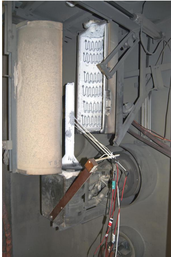
Figure 3-9 Setup of the mould for temperature measurements of tilt casting.
