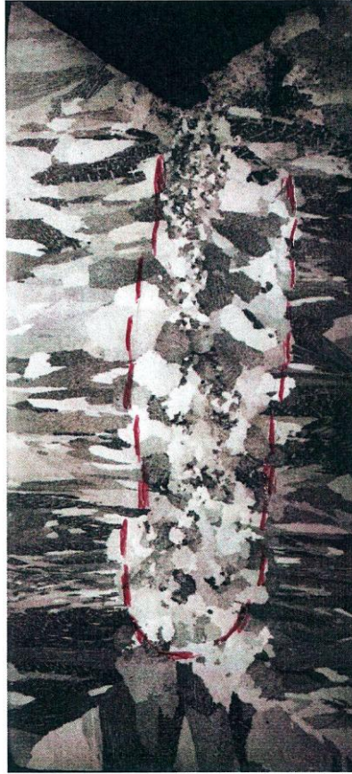
Figure 2-9 Macrograph of Al-4%Cu (wt. %) shows columnar to equiaxed transition, J. A. Spittle et al. 2006 [26].
