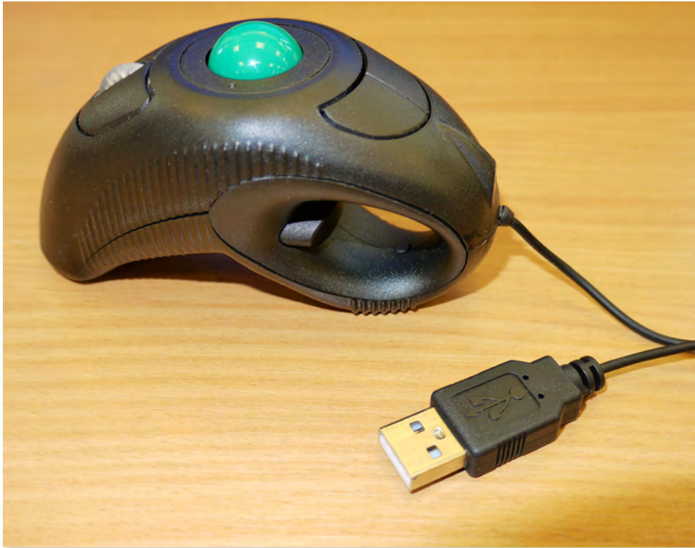
Figure 1.5.3 A trackball with scroll wheel and trigger mouse button
