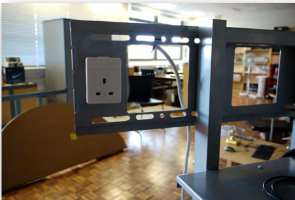
Figure 5.10 A single gang mains block mounted on the rear of the display mounting panel.
