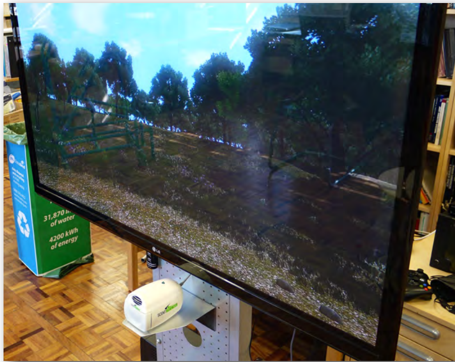
Figure 5.16 The Scentscape system fitted to the VR-I module during evaluation.
