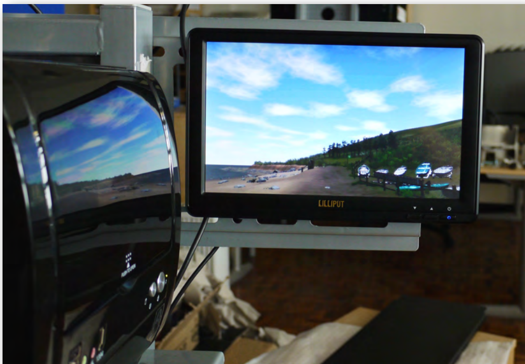
Figure 10.7 Lilliput USB display test fitted to the rear of the VR-I module.
