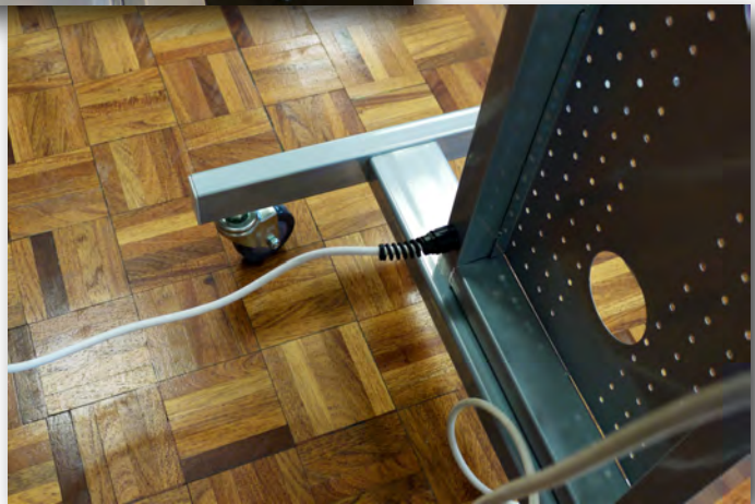
Figure 5.9 Cable from the mains block exiting at the base of the stand via a flexible cable gland.
