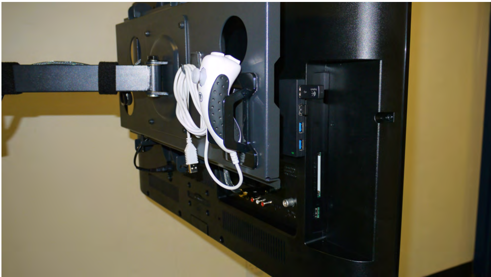
Figure 13.9 USB 3.0 Hub mounted to the display.
