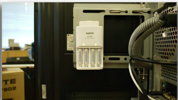
Figure 5.11 A battery charger installed during testing ensured that the audio system remained functional at all time.
