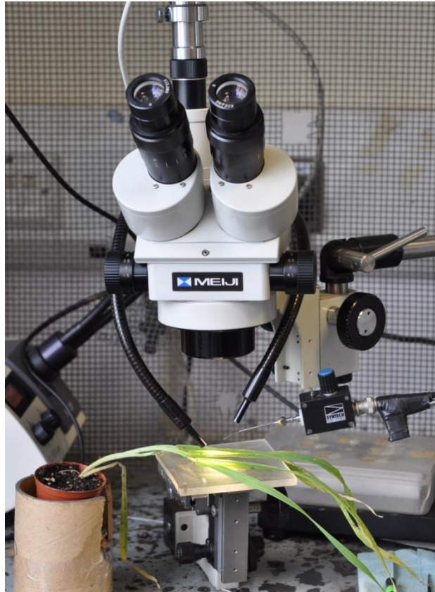
Figure 1-5 Stylectomy set-up showing microscope, light source and sharpened tungsten needle attached to micromanipulator.
