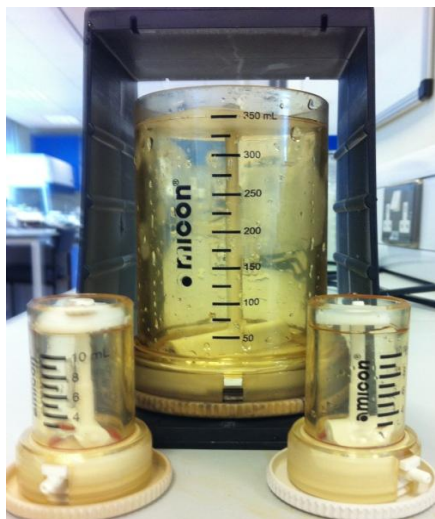
Figure 2.5: 350 mL and 10 mL Amicon stirred ultrafiltration systems used in the present study.
