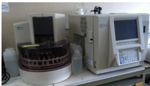
Figure 2.10: Shimadzu TOC-V CSH total organic carbon analyzer at the University of Birmingham.
