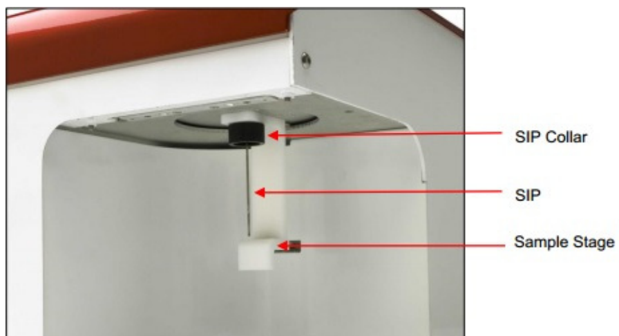
Figure 3-10 Sample introduction probe (SIP) and sample stage (Accuri C6 instrument manual)
