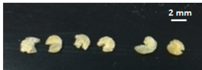
Figure 7-2 Typical optical image of CaP bead fractured by a diametrical compression test after being compressed with a 100 N load cell
