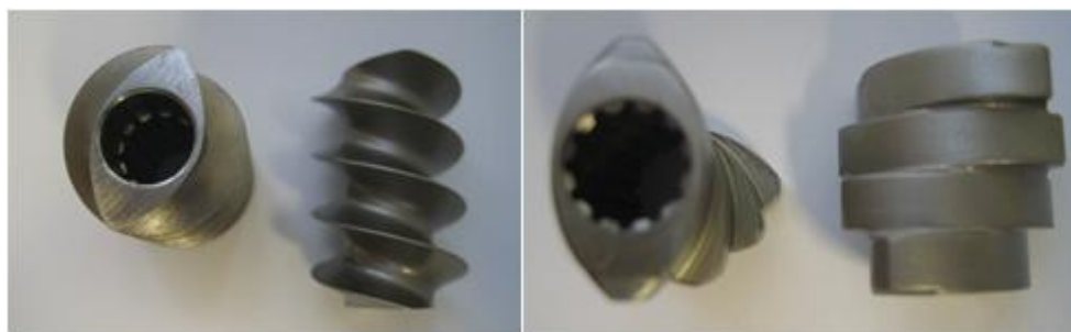
Figure 2.15: Types of screw elements. left: conveying right: mixing (30° forward)
