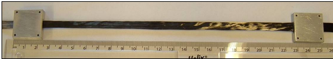
Figure 18: A carbon sample ready for Acoustic Emission testing.
