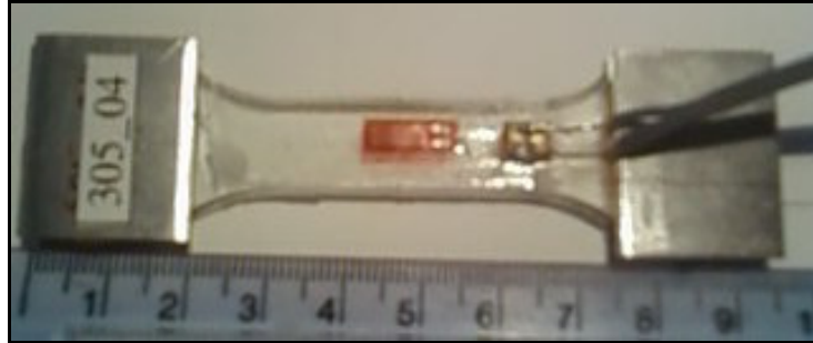
Figure 13: A cured Epo Tek 305 Resin sample with attached strain gauge.
