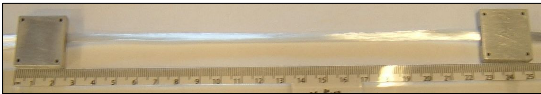
Figure 19: An uncoated E-glass sample ready for Acoustic Emission testing.
