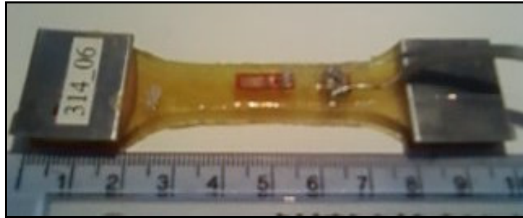
Figure 15: A cured Epo Tek 314 Resin sample with attached strain gauge.
