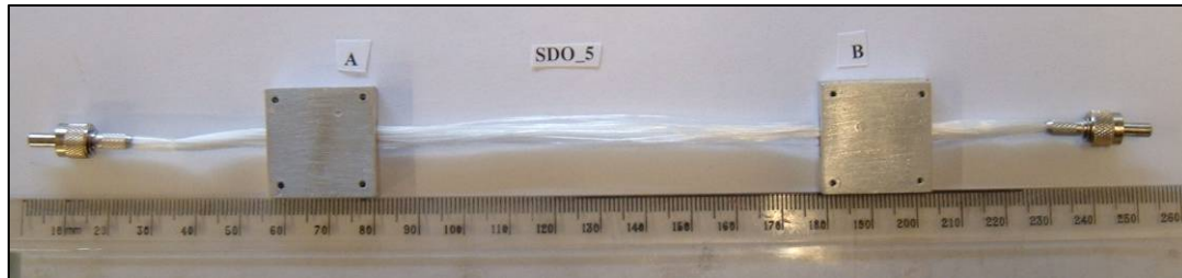
Figure 21: A small diameter optical fibre sample ready for self-sensing testing.
