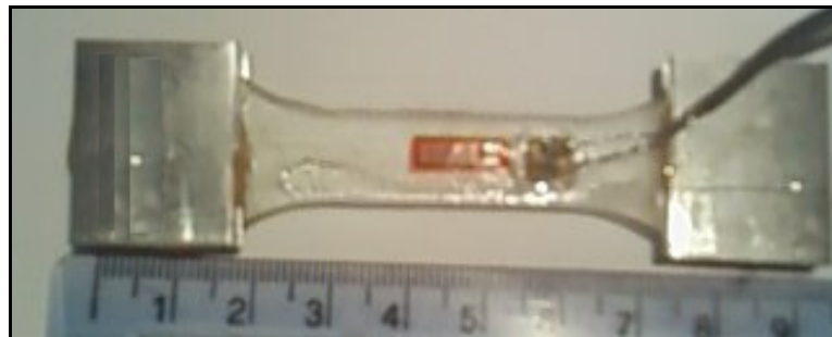
Figure 14: A cured Epo Tek 310M Resin sample ready for testing.
