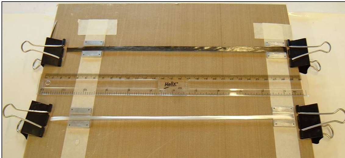
Figure 17: The setup used to fabricate carbon and uncoated E-glass samples for Acoustic Emission testing.
