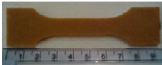
Figure 12: A cured Scotchweld Resin sample ready for testing.
