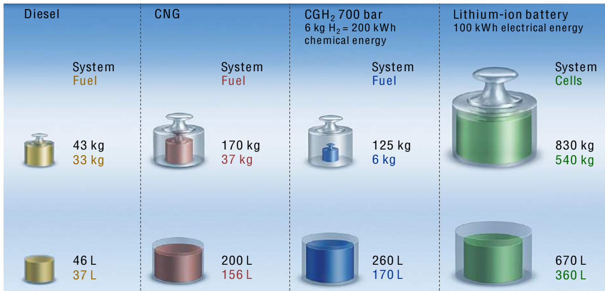
Figure 1.3 Weight and volume of energy storage materials and systems for a vehicle with a driving range of 500 km, where CNG = compressed natural gas, CGH 2 = compressed gaseous hydrogen (Brinkman et al. , 2012).
