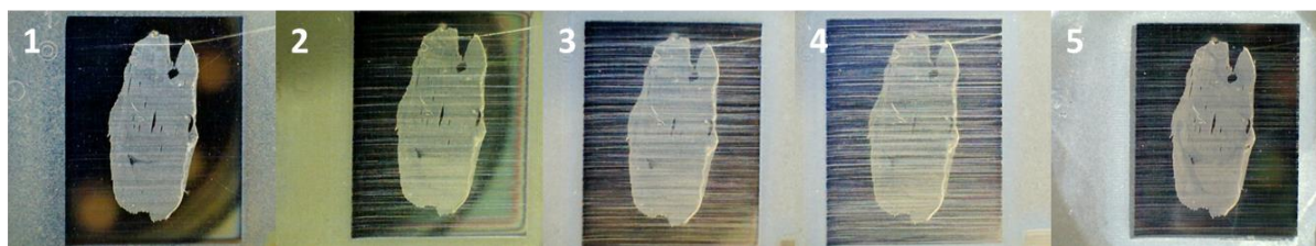
Figure 6.6. Image of build-up of unablated CHCA post analyses. Each image was taken after successive MALDI-MSI interrogations. Image five shows tissue section after 50 % ethanol wash step. Images correspond to data shown in Figure 6.5.
