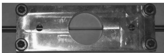
Figure 2–3 Photograph showing the quartz capillary used by Raber et al. [2006]
