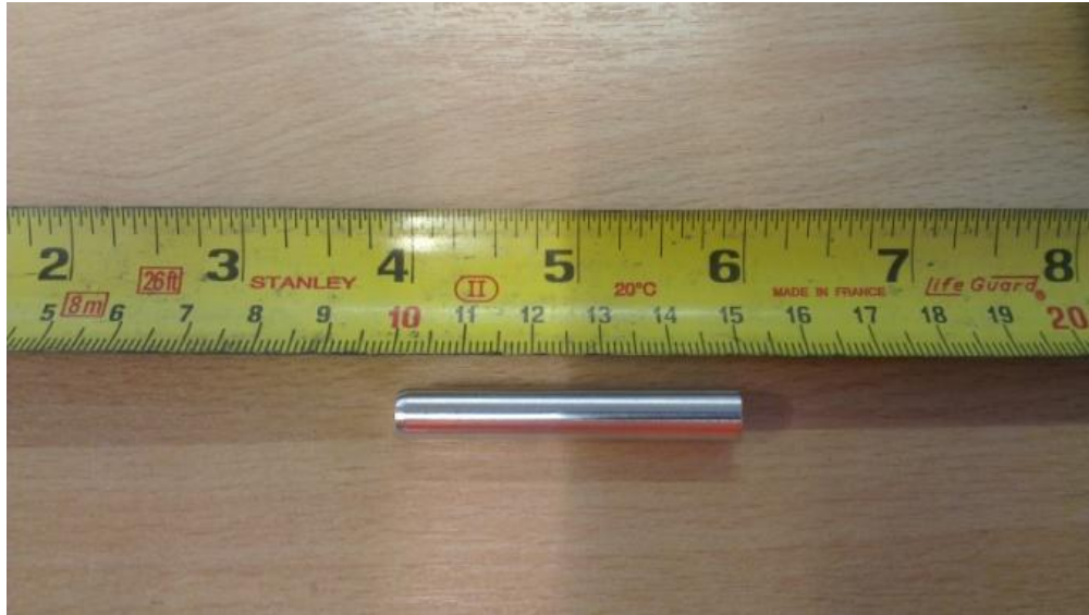
Figure 3.14 An Al sample used in the LECO H determination process, dimensions 8mm OD x 50 mm length.
