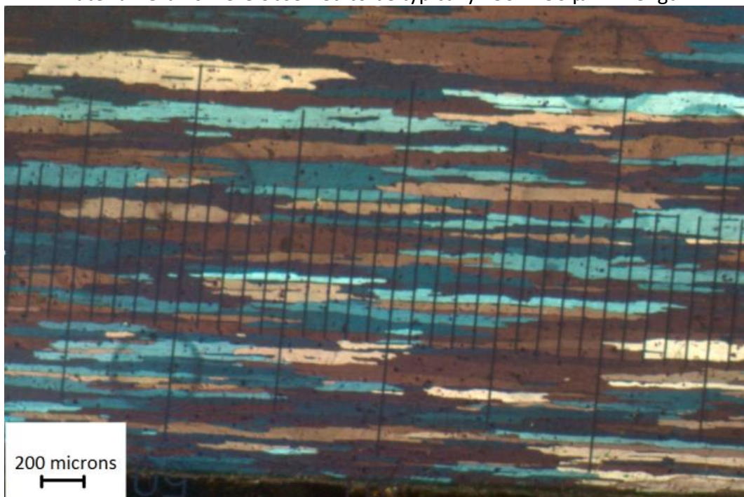
Figure 4.22 The near surface grain size of an anodised 7475 alloy plate from the edge of plate 1016502. Grains were observed to be typically 1000 - 2500 \mu\text{m} in length.
