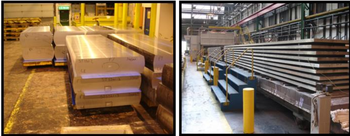
Figure 1.1 An example of DC cast Ingot that has been scalped. Figure 1.2 An example of rolled aluminium plate.
