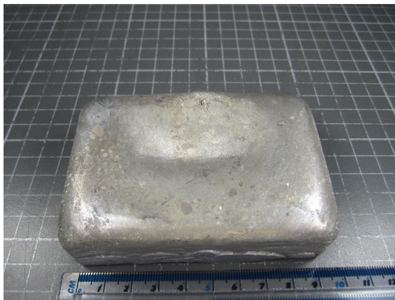
Fig. 3.2 Optical image obtained from the magnesium alloy ingot.
