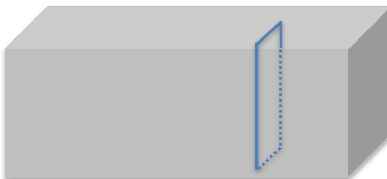
Fig. 3.3 Schematic representation of the sectioning of the specimens for microstructural characterization.
