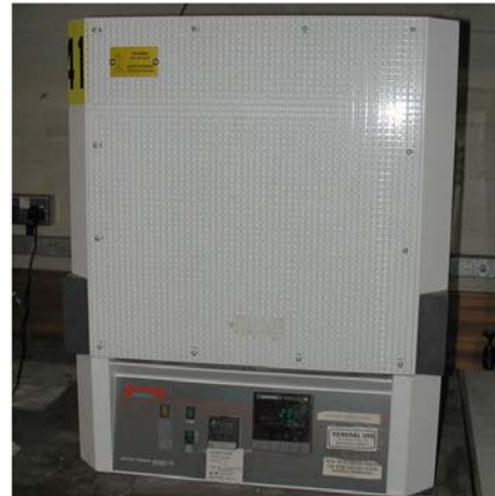
(d) Box furnace used for calcining powders and sintering compacted rods (<1700 °C) in air.
