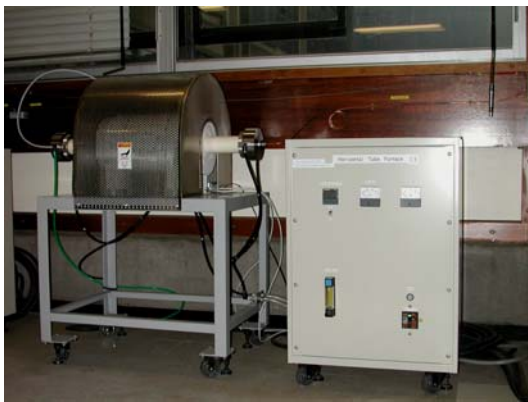
(c) Horizontal tube furnace used for calcining powders and sintering compacted rods (<1200 °C) in oxygen or air.
