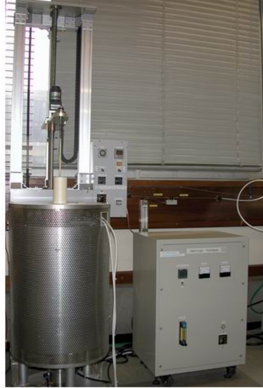
(b) Vertical tube furnace used for sintering compacted rods (<1750 °C).
