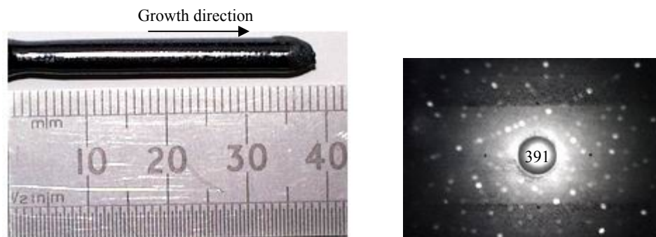
Fig.7.6. A typical \text{ErFeO}_3 single crystal grown using the four mirror image furnace (left), and a Laue diffraction taken from the cross section of the crystal (right) showing the high quality of the crystal with [391] as the growth direction.
