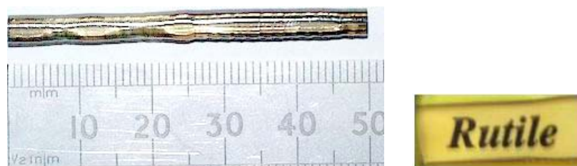
Fig.5.2. A typical as-grown rutile single crystal (left) and a view through a longitudinal section cut from such a crystal (right) to illustrate its transparency (the writing is below the crystal).
