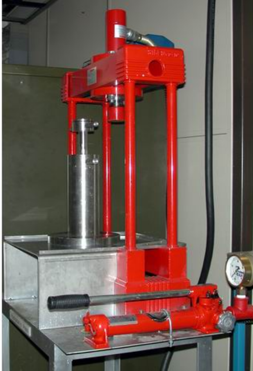
(a) Hydraulic press used for compacting starting powders into rods.
