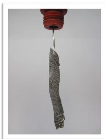
Figure 6 - Counter electrode affixed with a rubber stopper to maintain an airtight connection with the electrochemical cell
