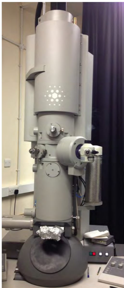
Figure 3.10: Schematic of TEM in operation alongside an image of the FEI Tecnai 20 TEM. Schematic modified from [12].
