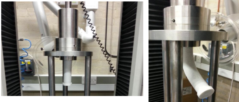
Figure 41 - Straight tube during extrusion (left) and the more commonly seen curved tube (right)
