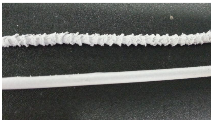
Figure 31 - Sodium aluminate paste extrudate, extruded at ram speeds of 50mm/min (top) and 1mm/min (bottom)
