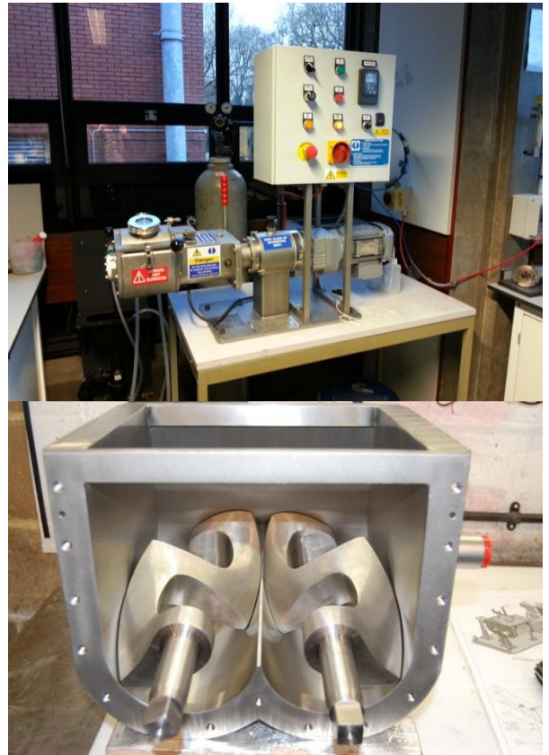
Figure 16 - Picture of Z-blade mixer used (top) and blade arrangement (bottom)
