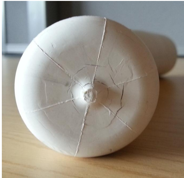
Figure 40 - Photo of cracks in closed end tube ( D = 0.05\text{m} )
