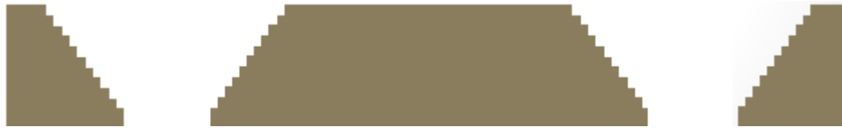
Figure 23 - Diagram of "steps" used to calculate pressure drop in tapered annulus
