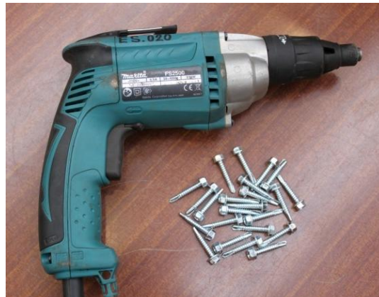
Figure 3-11: 5.5 × 32mm Tek screws and self-drilling machine
