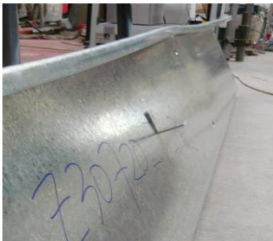
Figure 5-11: Permanent distortional buckling deformation
