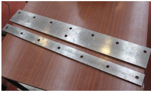
Figure 3-10: Steel plate with dimensions 100mm × 800mm × 10mm and 50mm × 800mm × 10mm
