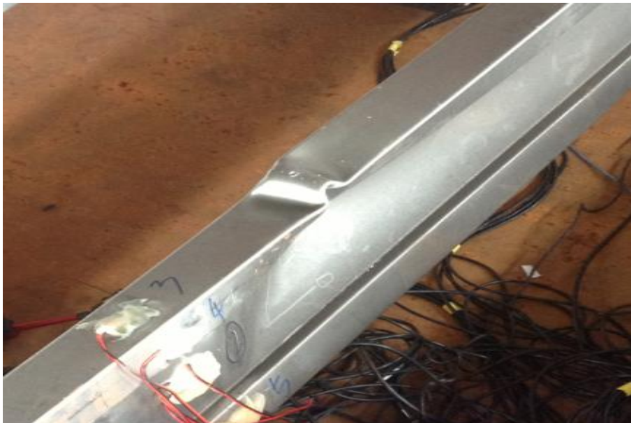
Figure 5-26: Local buckling of purlin \Sigma 30030 FD
