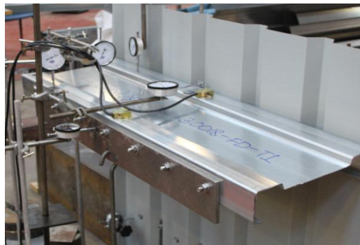
Figure 3-12: Multiple-point loads to simulate the uniformly distributed load
