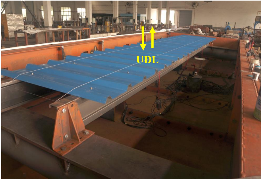
Figure 5-23: Overview of vacuum chamber test set-up
