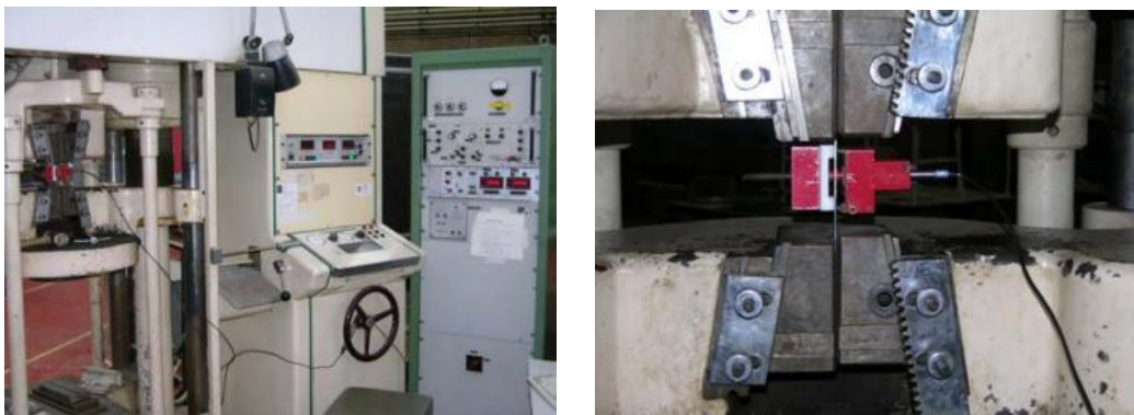
Figure A.1.1: Tensile testing machine Figure A.1.2: Sample steel coupon under testing
