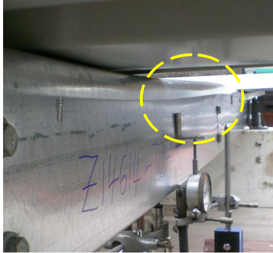
Figure 5-5: Distortional waves in flange-lip junction
