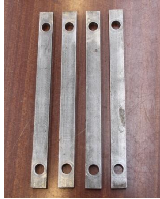
Figure 3-9: Four steel plates with dimensions 250mm × 20mm × 10mm
