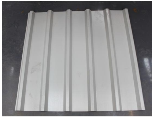
Figure 3-6: Sheeting with dimensions 1060mm × 1000mm × 0.7mm
