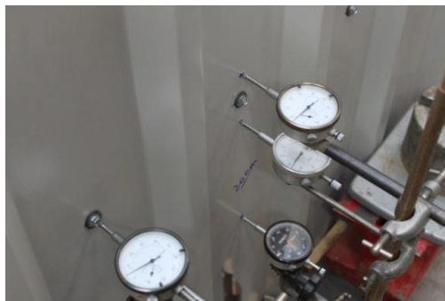
(a) Dial gauges placed at the rear side of the roof sheet
