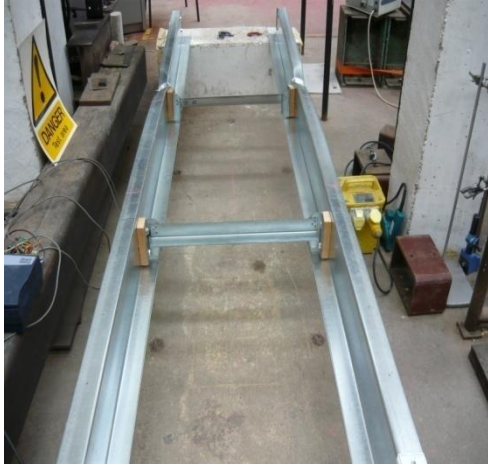
Figure 5-3: Anti-sag bars arrangement
