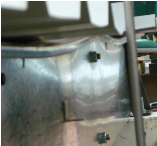
Figure 5-9: Distortional buckling waves
