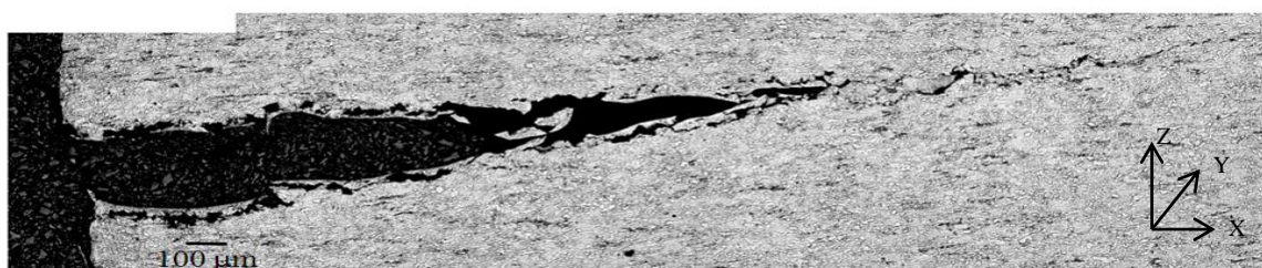
Figure 5.6. Optical microscopy image for the sectioned low blow (80 J impact energy) sample from the 16.8 mm strip in the longitudinal orientation showing a large ( \approx 4.2 mm length) split. The notch position is to the left of the image.
