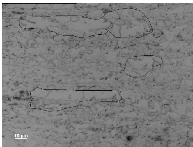
Figure 7.2. Optical micrograph of Steel X in the longitudinal orientation showing coarse grain patches (outlined).
