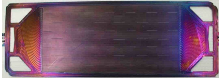
Figure 2.16 Treadstone Technologies Inc. coating on a Ford bipolar plate
