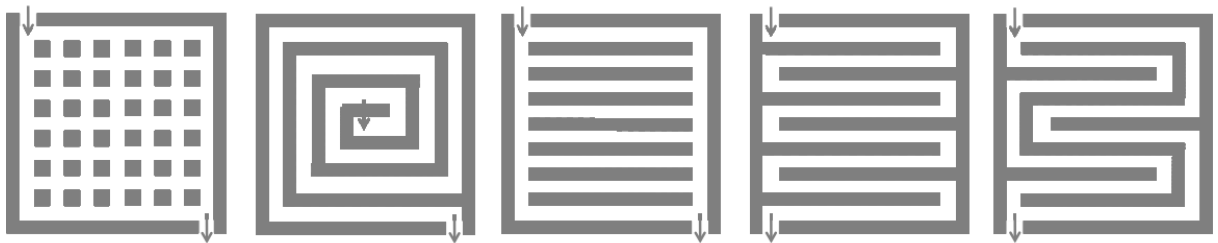
Figure 2.4 Typical flow field designs; grid/pin, spiral, straight-parallel, serpentine, and multiple serpentine
