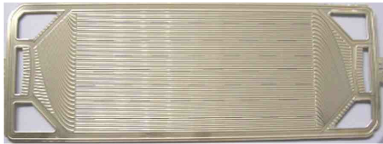
Figure 2.15 Daido Steel's Au Nanoclad ® coating on a Ford bipolar plate
