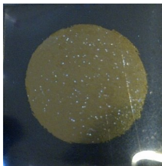
Figure 6.14 Photo of TiN+C coating after the potentiodynamic test showing the loss of the carbon topcoat and some pitting of the underlying substrate
