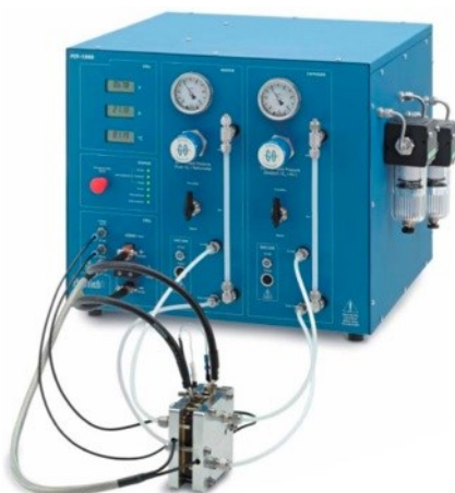
Figure 3.8 PaxiTech/Bio-logic FCT-50 Fuel Cell Test Station [204]
