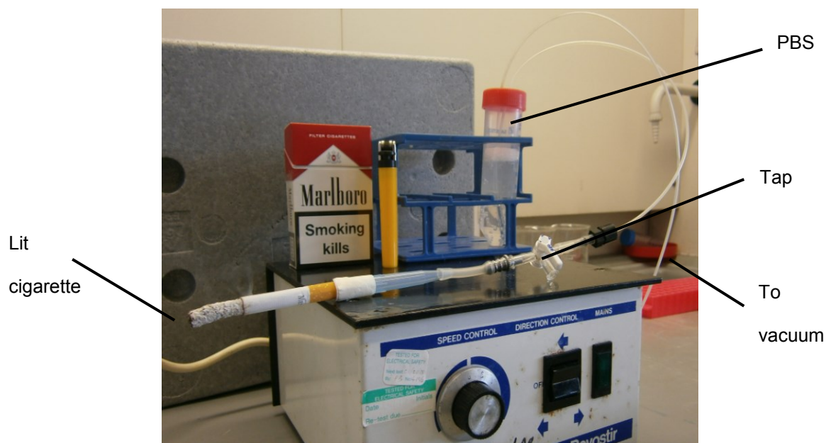
Figure 2.1 Generation of cigarette smoke extract. One Marlboro Red cigarette was lit in a fume hood for 10 minutes. The smoke was passed through a filter and collected by bubbling into 30ml of PBS at room temperature using a vacuum pump.
