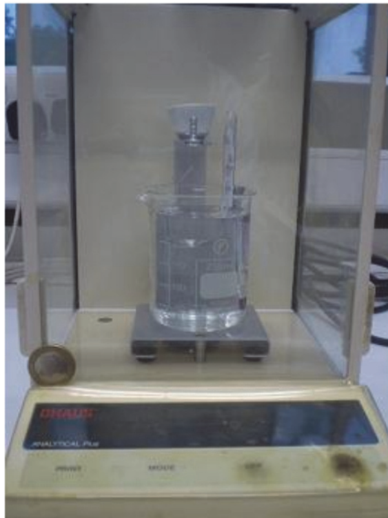
Figure 17 Photograph showing the equipment used to measure the density of the pultruded composites.
