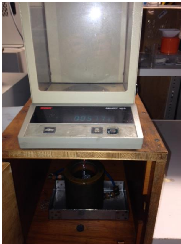
Figure 4.4.7. Ohaus Galaxy densitometer showing air and fluid measurement chambers.
