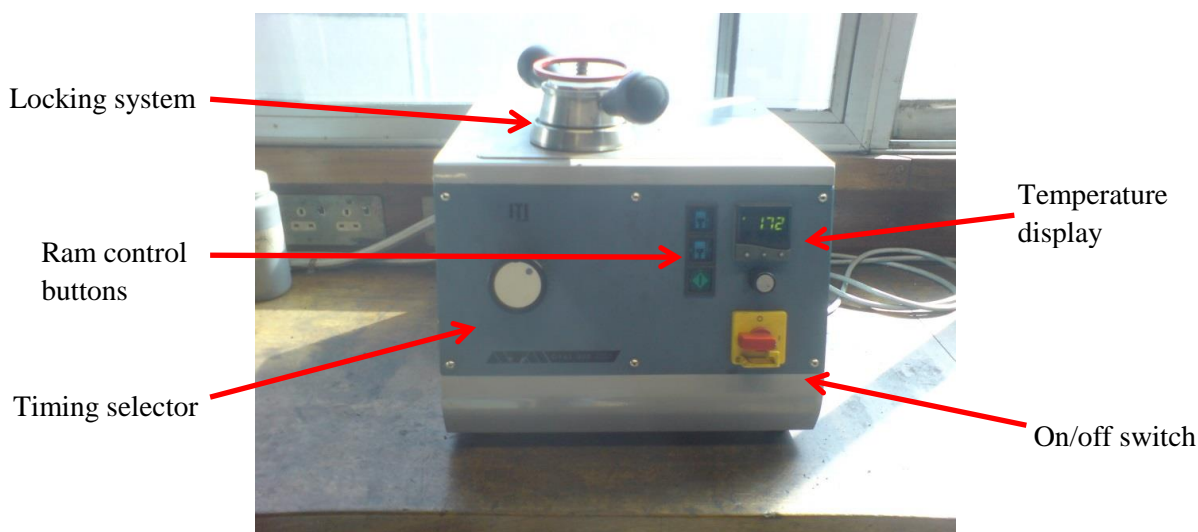
Figure 4.4.6. Opal 400 mounting press for mounting samples in Bakelite
