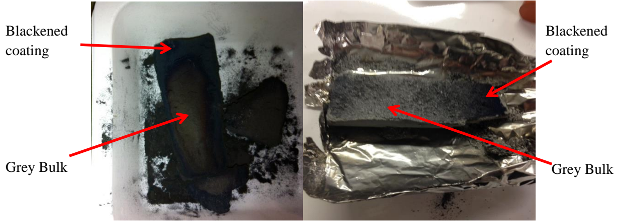
Figure 9.2. Appearance of sample as removed from the HDDR furnace, consisting of grey bulk material with a blackened coating
