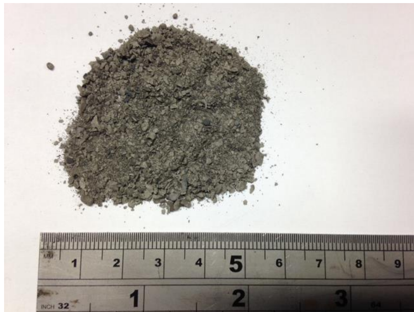
Figure 6.3. Photograph of hydrogen decrepitated powder before HDDR processing.
