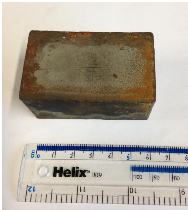
Figure 3.2.6. Corroded uncoated NdFeB magnet exposed to air for prolonged period of time
