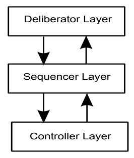
Figure 13: Three layers in 3T architecture for robotic control, adapted from [40]
