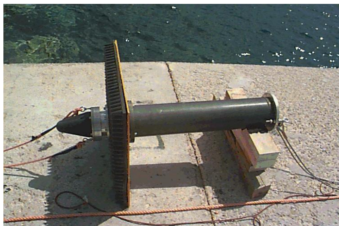
Figure 1.2: The receiving unit of the VERTLINK system. The baffle is mounted around the case facing the transducer
