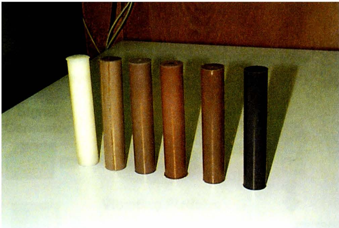
Figure 4.2: Loaded polyurethane samples (from left to right: glass microspheres, lead oxide in varying percentages, tungsten oxide)
