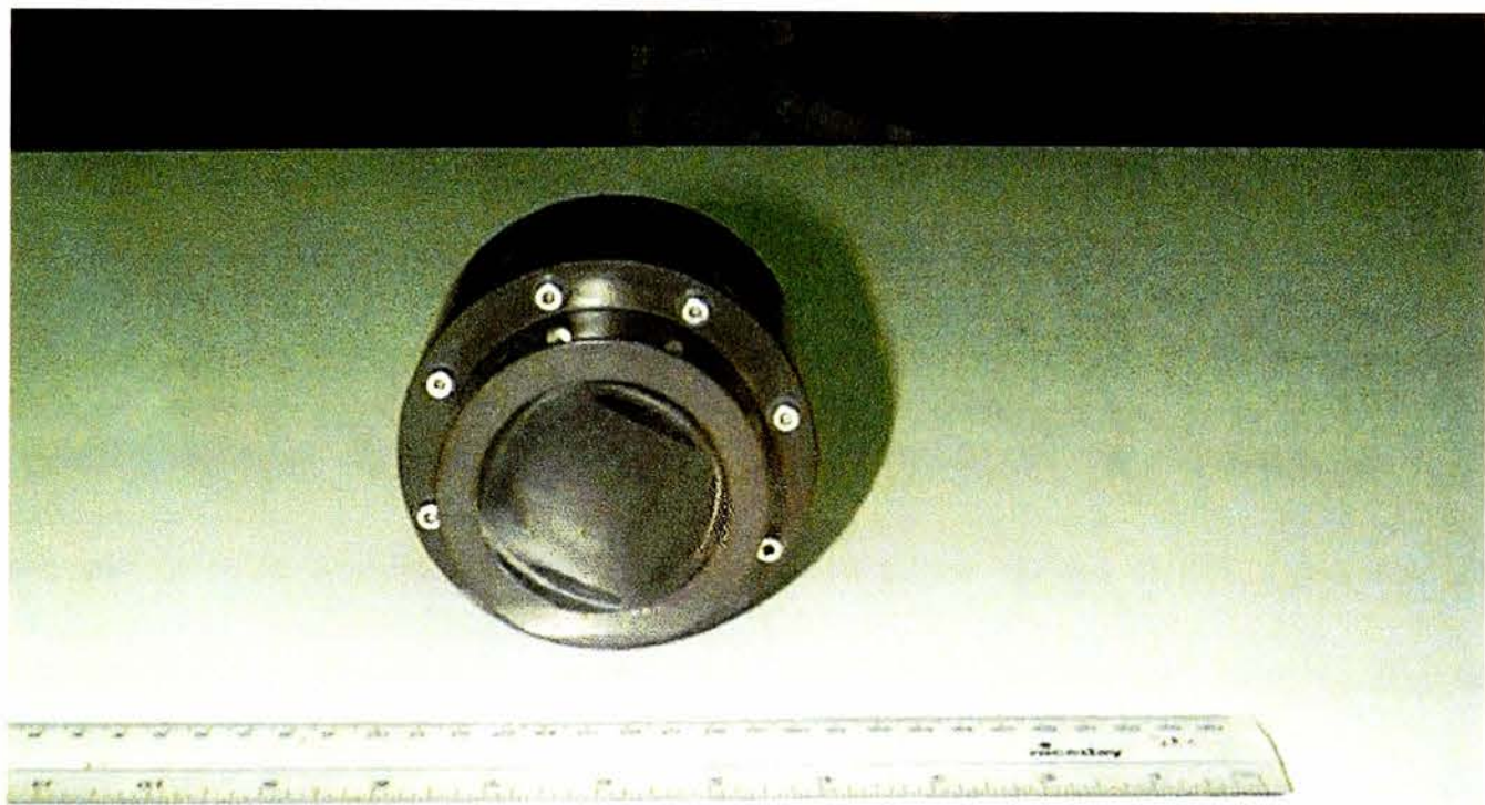
Figure C.11: The test parametric transducer (side view). The aluminium anodised body contains the matching transformers
