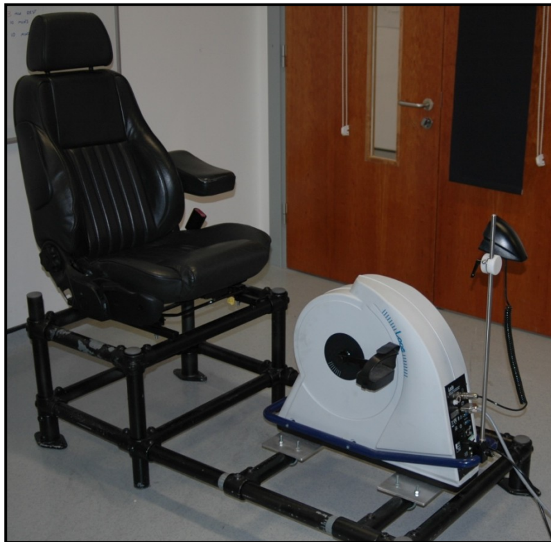
Figure 2.3 Customised electrically braked cycle ergometer
