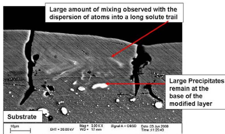
Figure 8.20 Backscattered SEM images (prepared by non-aqueous polishing to 1 \mu m surface finish) of microstructural cross-sections of solute dispersion by convection mixing and precipitates remaining at the base of the modified layer from electron beam surface melting on AA2024 with a high number of pulses per unit area (40) at 20 \mu s pulse duration and 2.5J.
