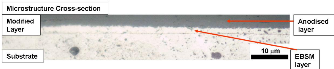
Figure 8.17 Uniform melt zone etched microstructure cross-section electron beam surface melted AA2024 at 4J, 5 \mu\text{s} pulse duration and 1 pulse per unit area, coupled with chromic acid anodising.
