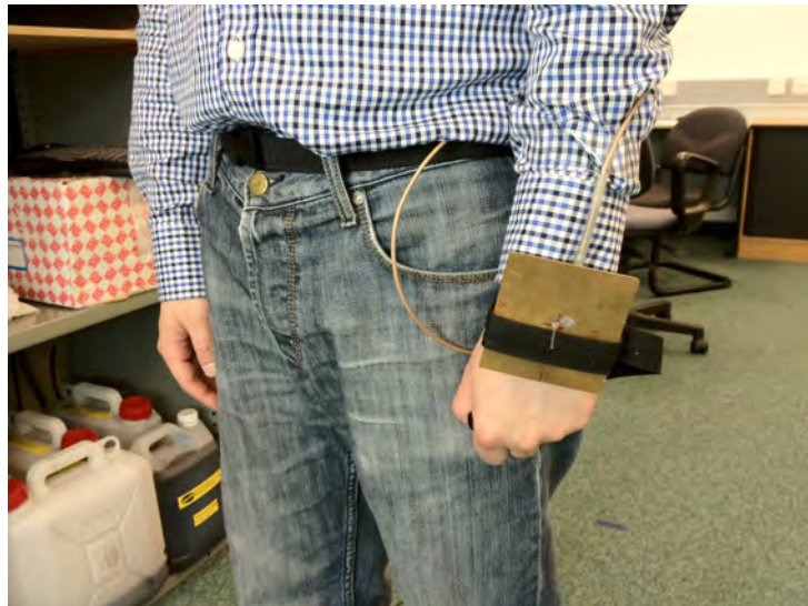
Figure 6.2: Monopole antenna on the wrist (2.45 GHz).
