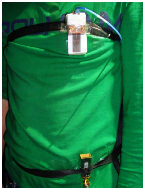
Figure 8.16: Belt-chest link using a printed Yagi-Uda and horn antennas.
