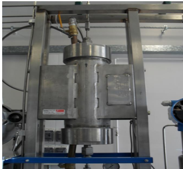
Fig.3.11. Condenser unit on a large-scale rig.
