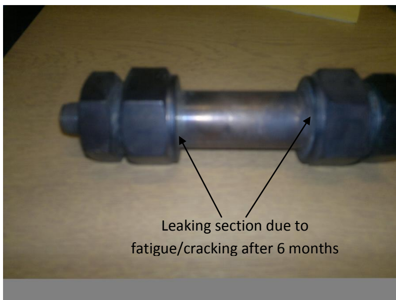
Fig.7.3. Small reactor with sign of fatigue due to fatigue and corrosion
