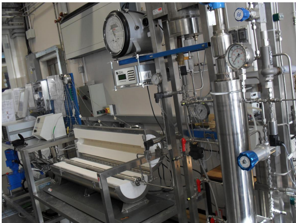
Fig.3.7. Image of the full process after construction (Note: separator unit in the foreground and reactor in the middle)
