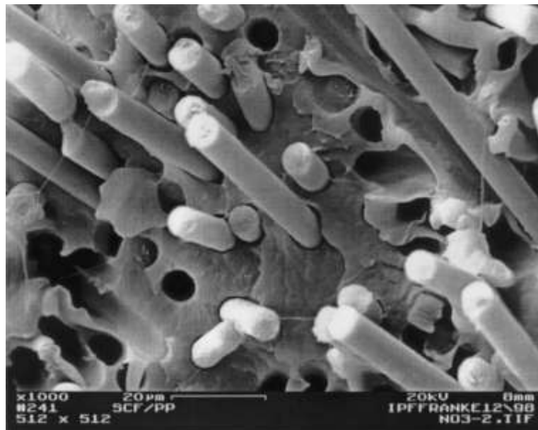
Figure 5 Scanning Electron Microscopy micrograph of tensile fracture surface of a short-carbon fibre polypropylene composite [32].
