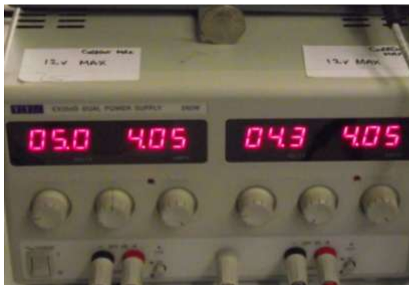
Figure 16 The power supply (EX354D Dual power supply) used to drive the fibre chopper.
