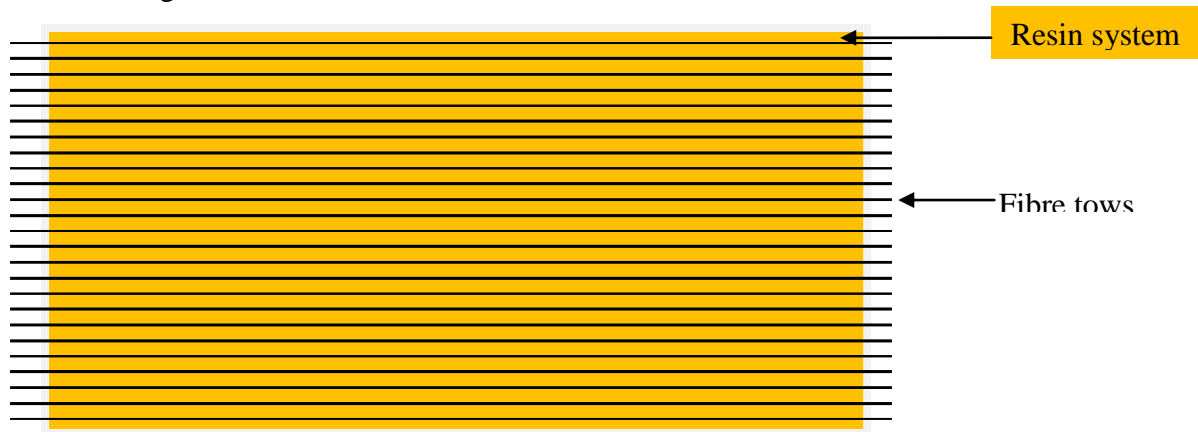
Figure 13 A schematic illustration of the placement of the fibre tows over the resin material.
